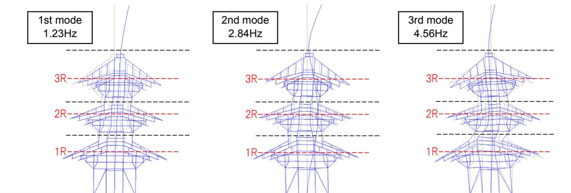
**Figure 8.** Modal shapes in sway motions reproduced with numerical model (Tower-1)
