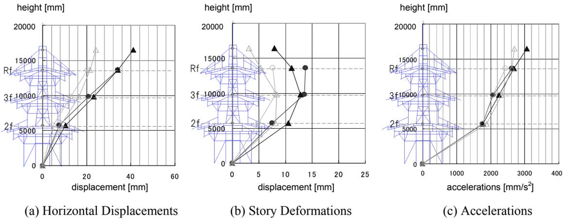
**Figure 11.** The maximum responses for seismic analyses (Tower-2)
