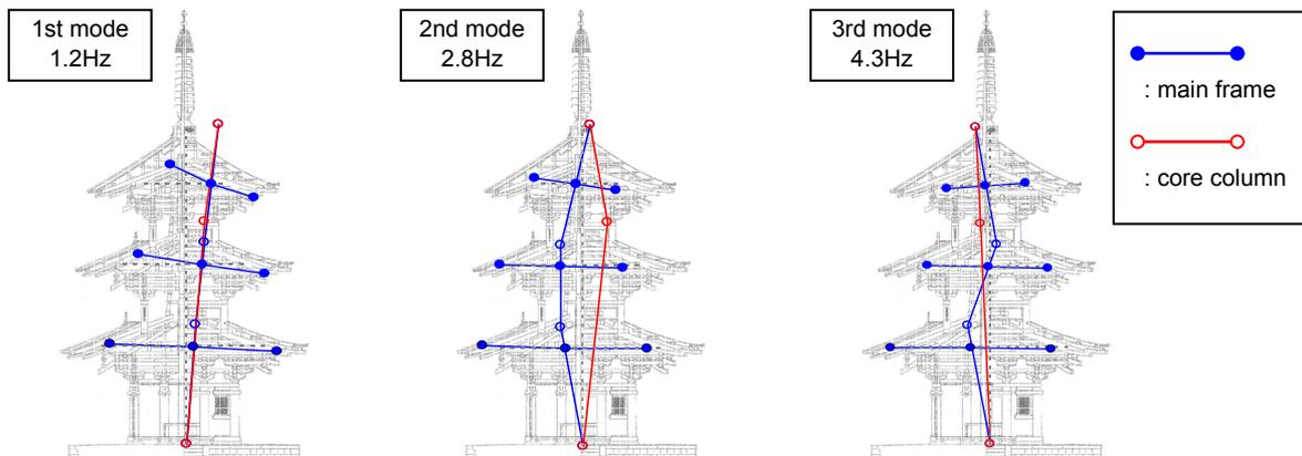
Figure 5. Modal shapes in sway motions identified by micro-tremor measurement (Tower-1)
