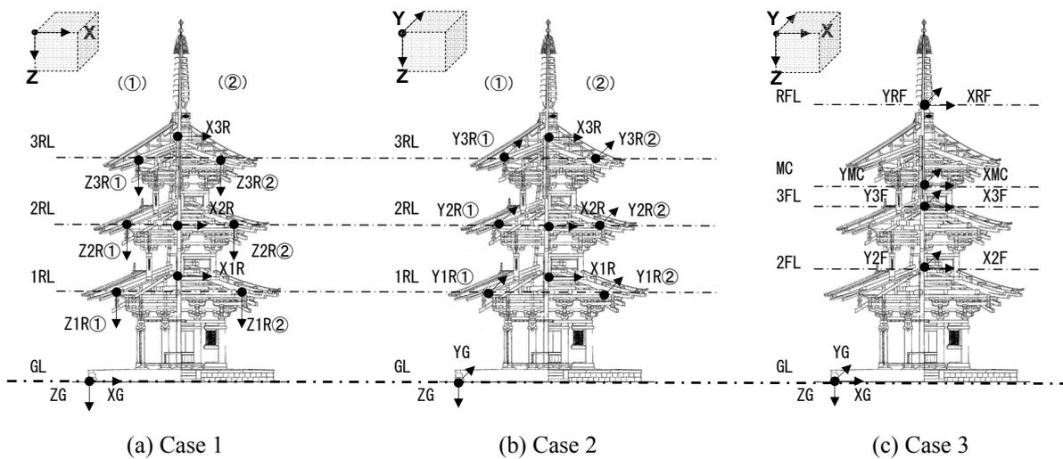
Figure 2. Pattern of allocation of the velocity sensors
