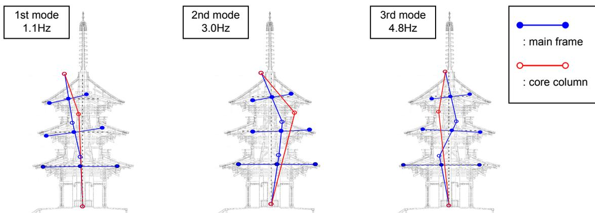
Figure 6. Modal shapes in sway motions identified by micro-tremor measurement (Tower-2)
