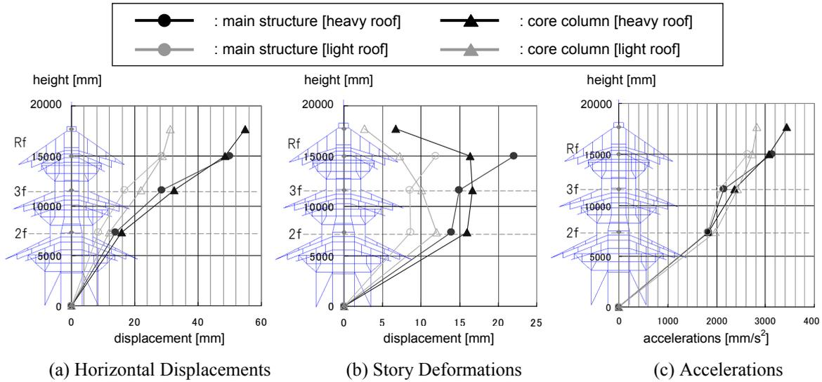
**Figure 10.** The maximum responses for seismic analyses (Tower-1)
