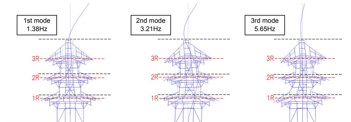
**Figure 9.** Modal shapes in sway motions reproduced with numerical model (Tower-2)
