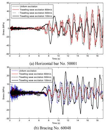
**Figure 4** Time-history of stress responses under different travelling wave excitations **Table 3.2** Peak stress responses under different earthquake excitations (Unit: MPa)
