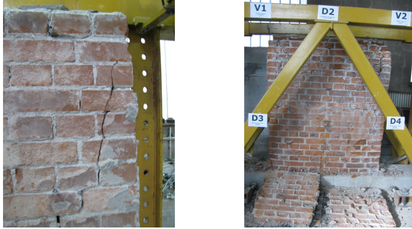
Figure 3.3. Experimental cracking pattern for strengthened masonry walls (masonry part)
