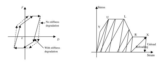
Figure 2. Hysteretic loop with stiffness degradation
