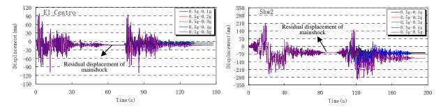
Figure 5. The response displacement of three-story RC frame structure under mainshock-aftershock sequence
