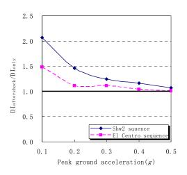
Figure.9 The ratio of Park and Ang's index of aftershock and mainshock only with PGA
