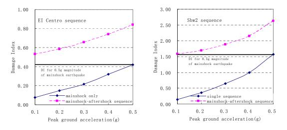
Figure.7 Park and Ang's damage index under mainshock-aftershock and mainshock only
