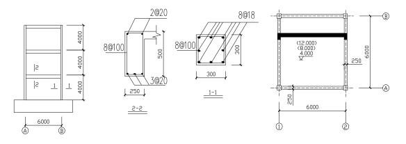
Figure 1. Dimensions of the three-story frame building
