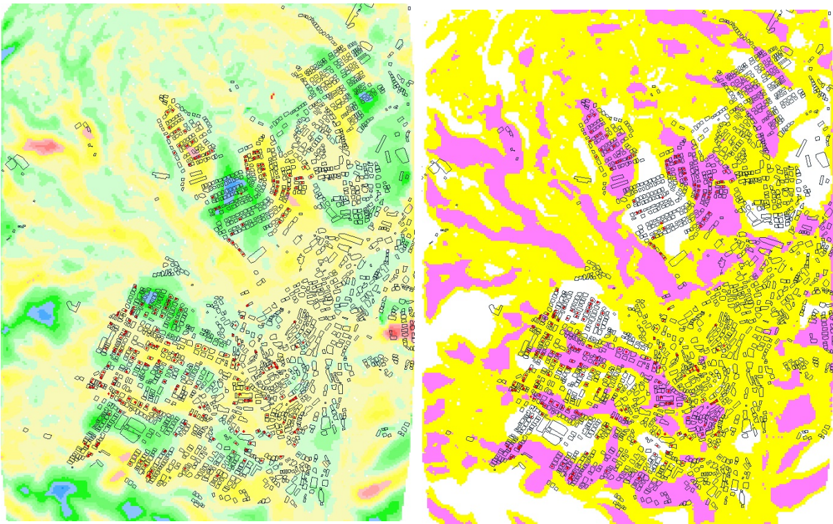
Figure 5 Fill-depth and cut-height coloring based on GIS estimation and tiled roof damage of houses at developed hill residential area (Koi-ue, Nishi Ward, Hiroshima City)
