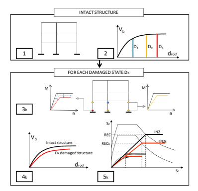
Figure 1. Flowchart illustrating the basic steps of the method for framed structures
