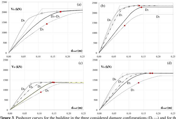
Figure 3. Pushover curves for the building in the three considered damage configurations  $(D_{1,2,3})$  and for the intact structure  $(D_0)$ : cases MAX (a), MAY (b), MOX (c) and MOY (d).
