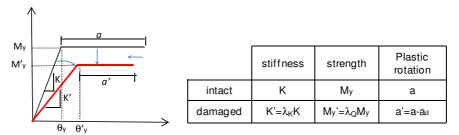
Figure 2. Modeling criteria for the damaged plastic hinges (adapted from (FEMA, 1998a))
