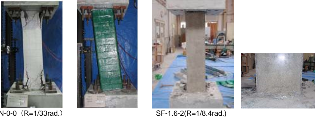
Photo 1. Crack patterns of concrete columns
