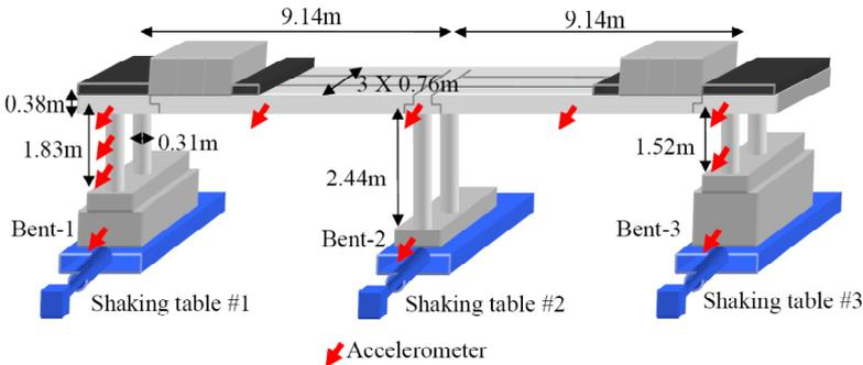
Figure 2.1. Schematic view of the model and sensor layout
