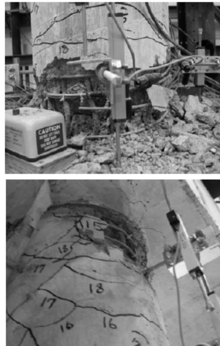
**Figure 2.4.** Damage observed on the lower and upper portion of Bent-3 after T-19
