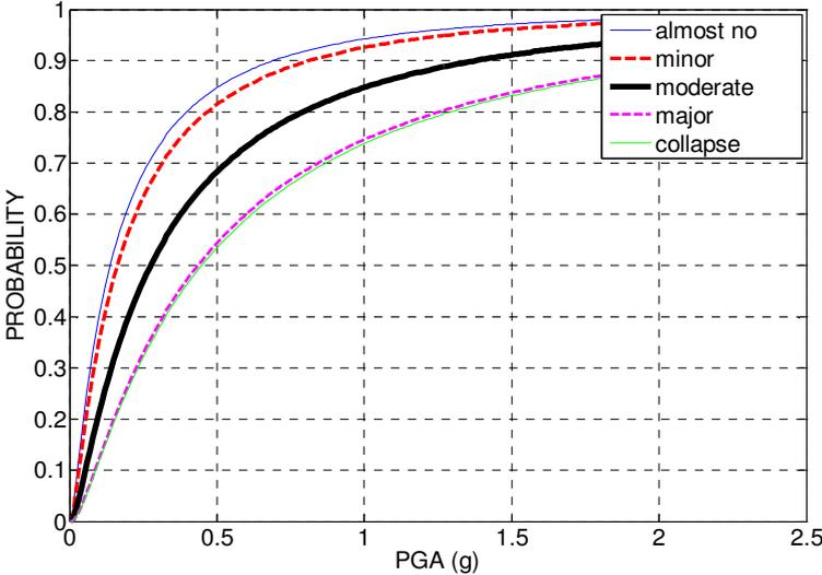
**Figure 5.1.** Fragility curves for undamaged structure
