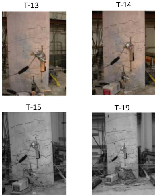
**Figure 2.3.** Damage observed on Bent-1 after each test
