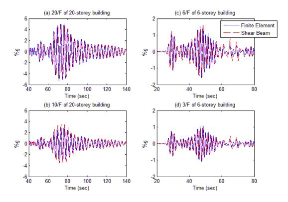
**Figure 5.** Comparison of responses from finite element models and shear beam models for the buildings in I-710/91 assuming a M 6 in San Bernadino with dip= 90°, rake= 180°, and strike = 120°. (a) Response at 20/F of 20-storey building; (b) Response at 10/F of 20-storey building; (c) Response at 6/F of 6-storey building; (d) Response at 3/F of 6-storey building
