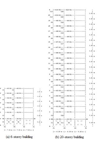
Figure 3. Finite element models of the 6-storey and 20-storey buildings
