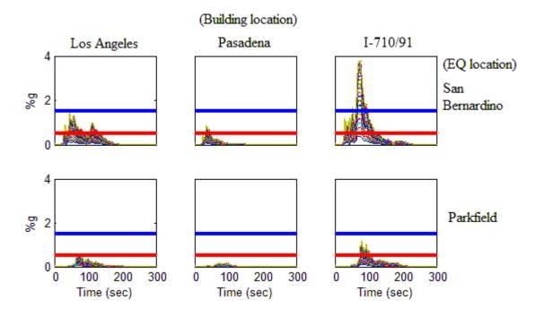
**Figure 6.** Seismic shaking level for 20-storey building. 20 curves on each plot correspond to different floor acceleration responses. (Red line: threshold for minor shaking; Blue line: threshold for moderate shaking)
