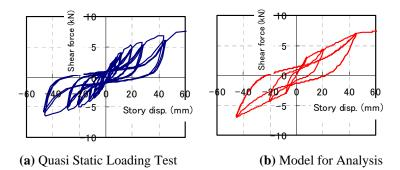
Figure 4.3. Force-Displacement Relationships and Non-linear Hysteresis Models of Nailed Plywood Panels
