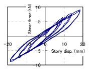
Figure 5.1. Measured Force - Displacement Relationship of a Frame with K-braced Dampers under Quasi-static Loading Test
