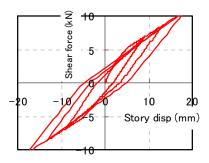
Figure 4.5. Non-linear Hysteresis Model of the Frame with K-braced Dampers by Push Over Analysis
