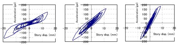
(a) Wall length ratio of damper=0%(K<sub>1</sub>=3.48, K<sub>2</sub>=3.27 kN/cm) (**b**) Wall length ratio=50% (K<sub>1</sub>=8.37, K<sub>2</sub>=4.88 kN/cm) (c) Wall length ratio=100% (K<sub>1</sub>=13.25, K<sub>2</sub>=6.48 kN/cm)
