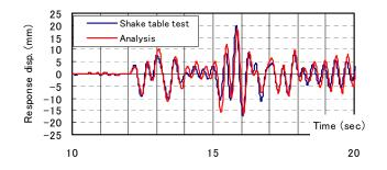
Figure 5.5. Response Displacements of the Frame with K-braced Dampers by Analysis and Shaking Table Test (JMA Kobe NS)
