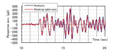
Figure 5.6. Response Accelerations of the Frame with K-braced Dampers by Analysis and Shaking Table Test (JMA Kobe NS)
