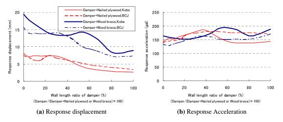
Figure 5.9. Relationship between Response of Frame and Wall Length Ratio of Damper
