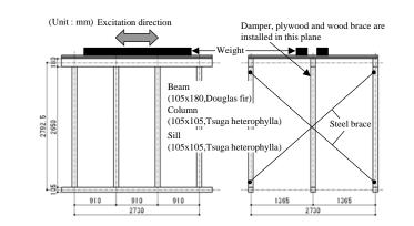
Figure 3.1. Elevations of the Three Wood Frames for Shaking Table Tests
