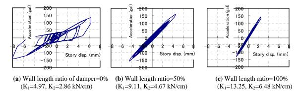
Figure 5.7. Response of the Frame with Dampers and Nailed Plywood Shear Panels under JMA Kobe Motion (W=22.295kN, Input=70.98gal)
