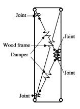
Figure 4.1. Schematic Models of Frame with Dampers for Response Analysis
