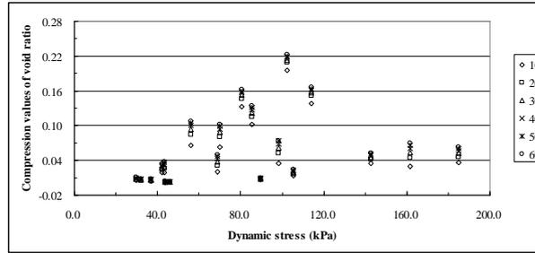
**Figure 2.4.** Relationship between dynamic stress and compression value of void ratio of untrimmed samples of unsaturated loess
