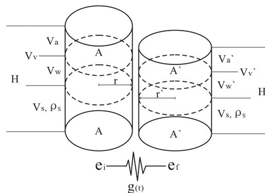
**Figure 2.3.** Ideal model for deformation analysis of three phases of air, water and solid of unsaturated loess
