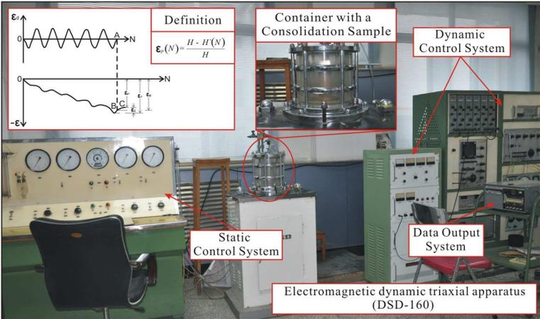
**Figure 2.1.** Laboratory panoramic view of dynamic triaxial test and definition of dynamic residual strain of unsaturated loess
