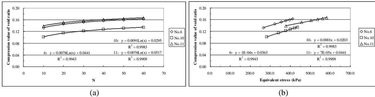
**Figure 2.5.** Examples of relations between compression value of void ratio and loading times of dynamic stress ( $N$ )/equivalent stress ( $f(\sigma_d)$ ) for single untrimmed sample of unsaturated loess
