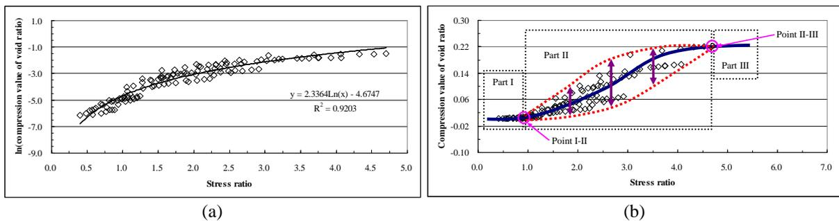
**Figure 3.2.** Empirical relationship and essential characteristics of void dynamic deformation of untrimmed samples of unsaturated loess
