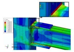
Figure 3.2. The von Mises stress distribution in specimen RC1
