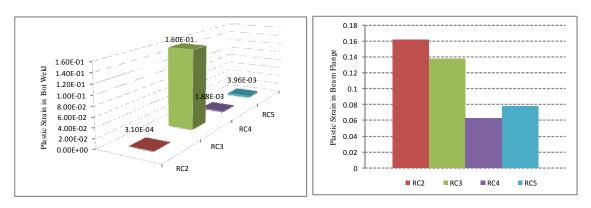
(a) (b) Figure 3.10. Max plastic strain of specimens; (a) bottom weld (b) beam flange
