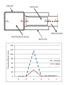
Figure 3.3. Strain response for specimen RC1
