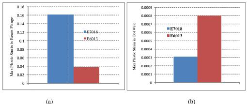
Figure 3.7. Maximum plastic strain: (a) beam flange (b) bottom weld
