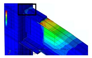
Figure 3.9. The plastic strain distribution in specimen RC3
