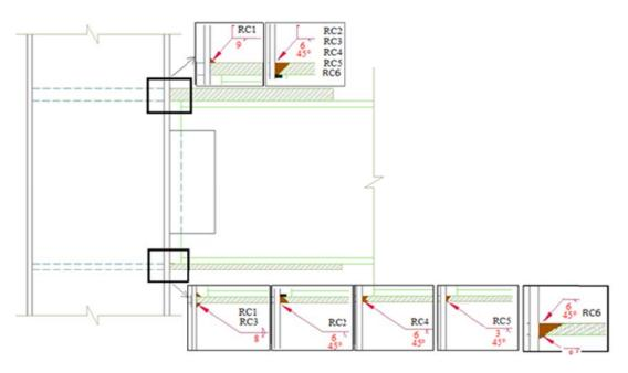
Figure 3.1.Geometry and weld types employed to join the flange plate to column
