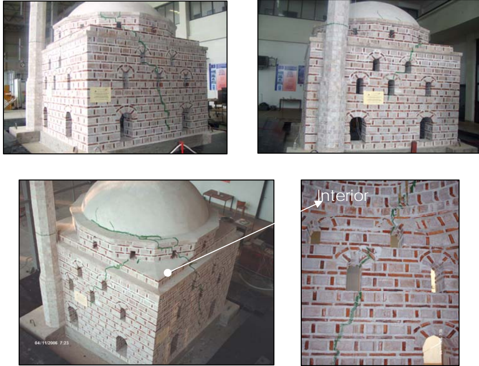
Figure 3.4 Damage to the model after phase 1 testing
