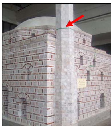
Figure 3.3 Horizontal crack at the base of the minaret
