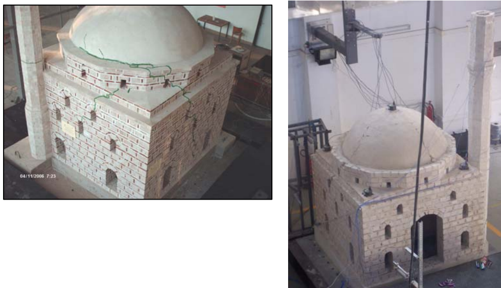
Figure 5.2. Comparison of damage distribution of the models (1/6 th scale model on the left, 1/10 th scale model on the right)
