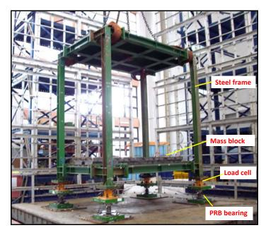
Figure 6. Test setup of the PRB-isolated steel frame.
