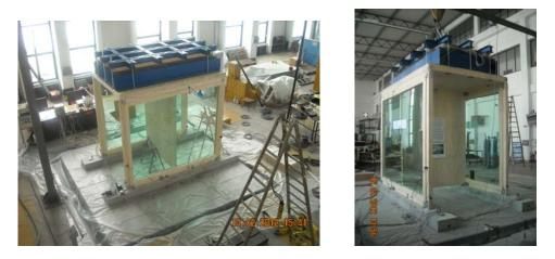
Figure 2. Loaded and instrumented model ready for testing
