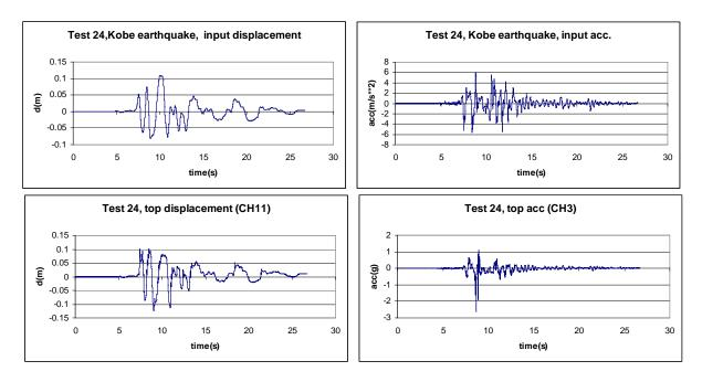
Figure 8. Input motion and response of the model, Kobe earthquake, test 24
