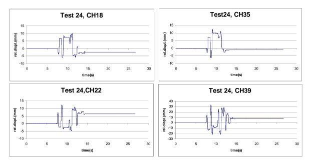
Figure 11. Slipping between the glass and the wooden frame during the Kobe earthquake, test 24
