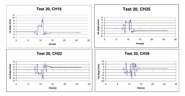
Figure 10. Slipping between the glass and the wooden frame during the Kobe earthquake, test 20
