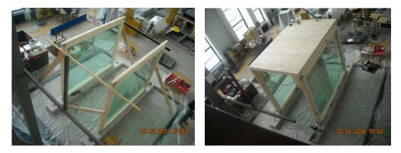
Figure 1. Model assembling - fixing of the two composite panels (left), completed model (right)
