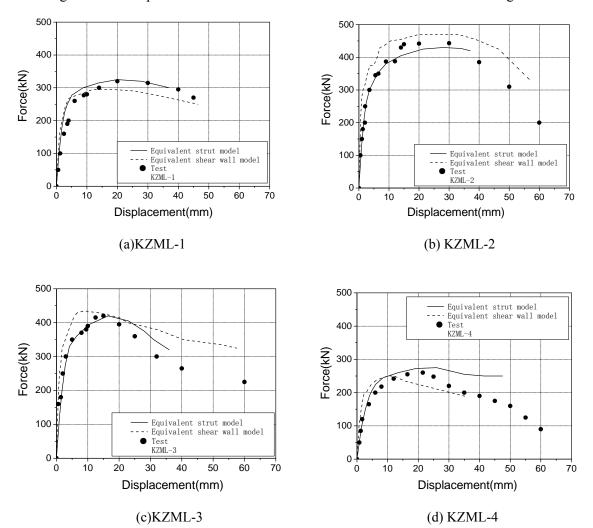
Figure 7. Force-displacement relation curves
