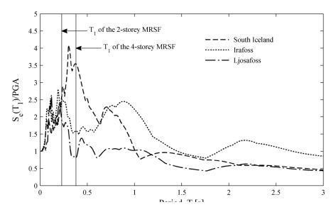
Figure 1. Elastic total acceleration response spectra for records
