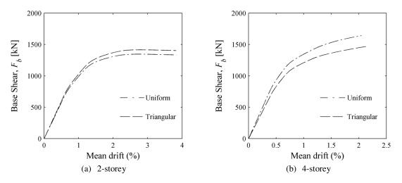
Figure 2. Capacity curve with different lateral load pattern for 2- and 4-storey
