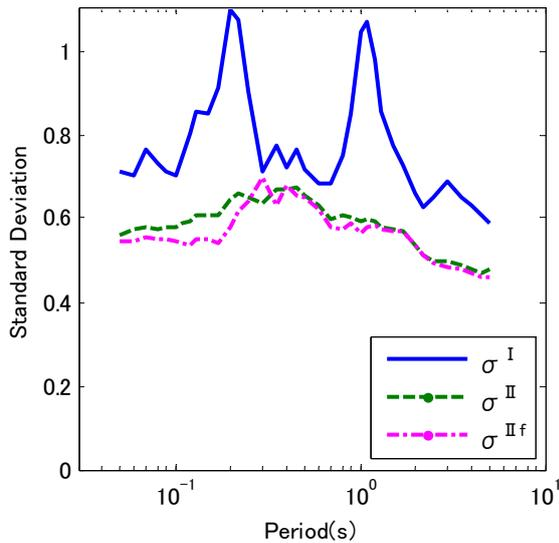
**Figure 3.4.** Standard Deviation of Sa of the Aftershocks Corrected for the Regression Equation
