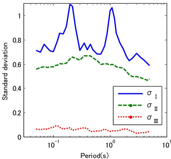
**Figure 2.2.** Standard Deviation of  $S_a$  of the Aftershocks
