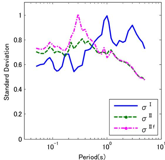
**Figure 3.5.** Standard deviation of Sa of the Shocks for Consideration Corrected for the Regression Equation
