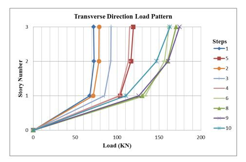
Figure 2.3. Transverse direction load pattern.
