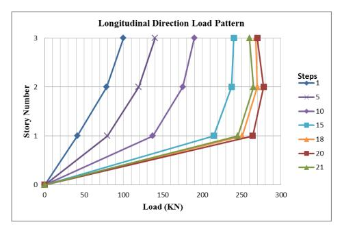
Figure 2.2. Longitudinal direction load pattern.
