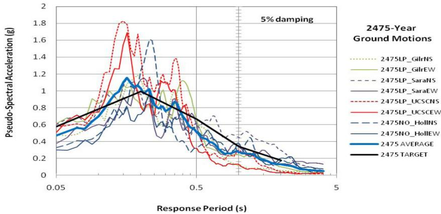
**Figure 4.** Response Spectra of Selected (Unscaled) Ground Motions (2,475 yr)
