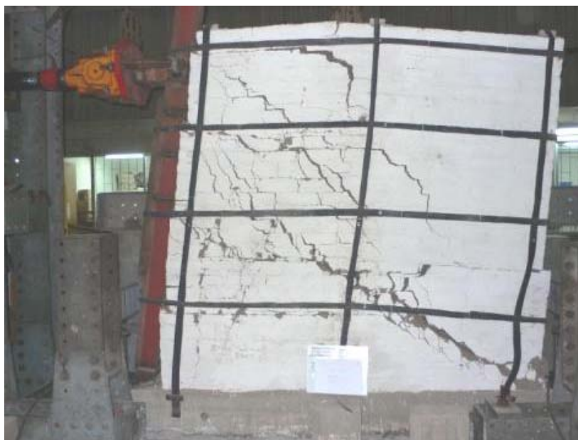
Figure 5. Even though subject to a large lateral displacement the wall was still able to resist load
