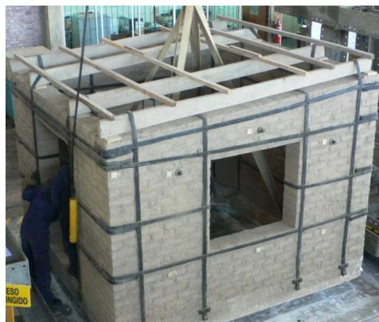
Figure 4. The adobe test module on the shaking table.
