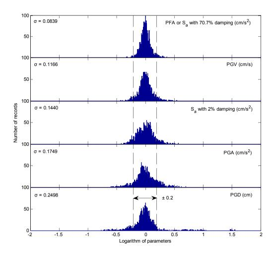
Figure 5.1. Comparison of performance of PFA, PGA, PGV, PGD and S<sub>a</sub> in collapse prediction, the intensity measures are normalized by their geometric mean values and plotted in log scale.
