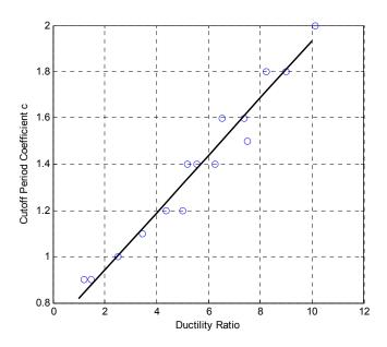
Figure 3.1. Regression model of cutoff period coefficient c
