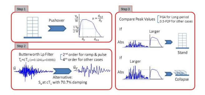
**Figure 1.1.** Procedure of prediction (T<sub>1</sub>-fundamental period, T<sub>c</sub>-cutoff period of Butterworth filter, c-developed coefficient which depends on the global ductility and ranges between 0.9 and 2.0)
