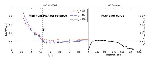
**Figure 2.1.** Example of minimum collapse PGA in sinusoidal ground motions for a US code six-story steel building (U6P) is shown on the left. The pushover curve is shown on the right. A common vertical axis is used for both panels.
