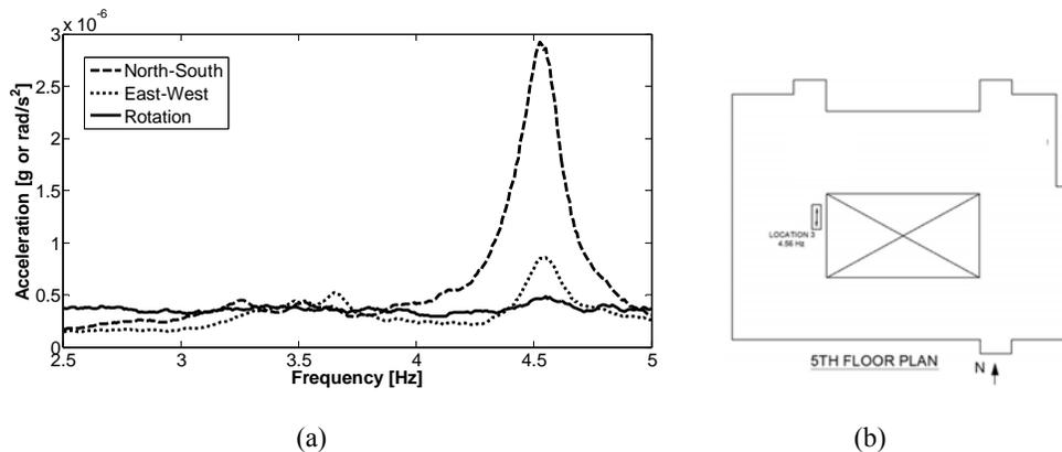
Figure 6.1 (a) Mode 3 FFT; (b) Mode 3 shaker location/orientation
