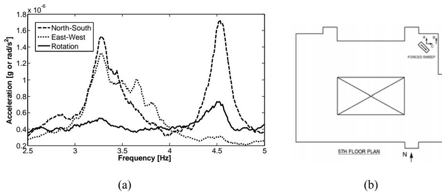
Figure 4.1. (a) Mode 1 FFT; (b) Mode 1 shaker location/orientation
