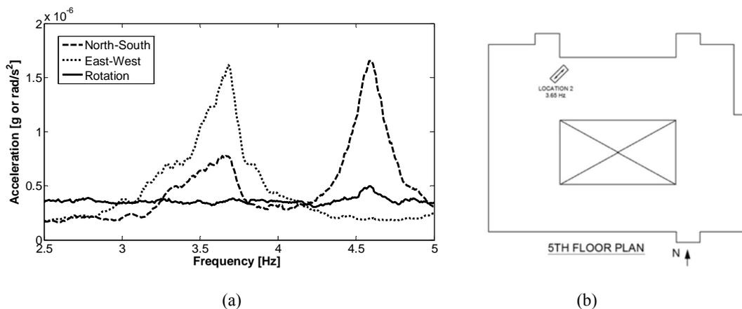
**Figure 5.1** (a) Mode 2 FFT; (b) Mode 2 shaker location/orientation
