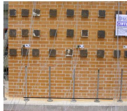
**Figure 3.4** Hairline crack between the solid walls and the base plate of the mock-up
