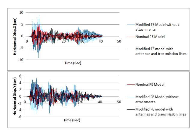
**Figure3.2.** Horizontal displacements of the mast at cable cluster elevation #1 (top cluster) along the X (along input) and Y (transverse to input)
