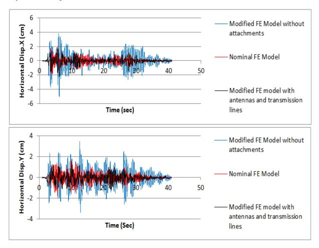
**Figure3.1.** Horizontal displacements of the mast at cable cluster elevation #6 (bottom cluster) along the X (along input) and Y (transverse to input)
