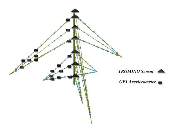
Figure 2.2. Location of the sensors on the tower
