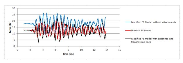
Figure 3.3. Axial tension in a typical cable of Cluster #1 aligned with the input ground motion.
