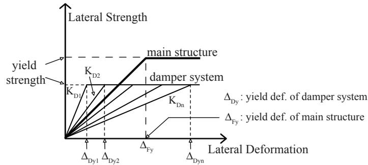
**Figure 1.1.** Schematic restoring force of main structure and dampers
