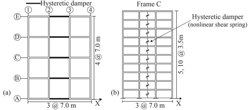
**Figure 2.2.** Analyzed R/C frames with hysteretic dampers: (a) typical plan and (b) elevation
