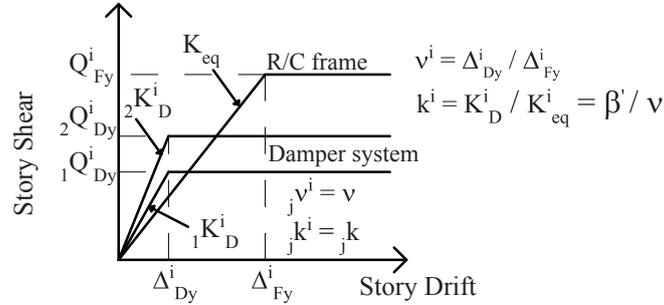
**Figure 2.3.** Story shear versus story drift relationship under the 'constant yield story-drift ratio' scheme
