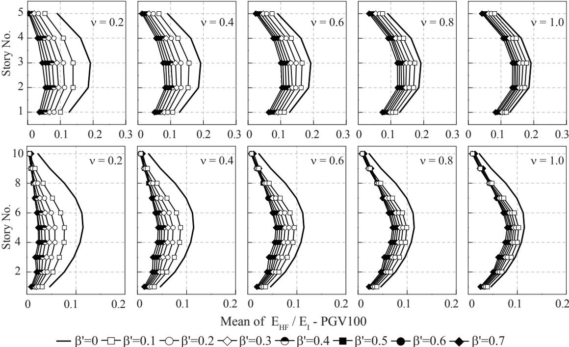
**Figure 4.4.** Participation of R/C frame into total input energy dissipation
