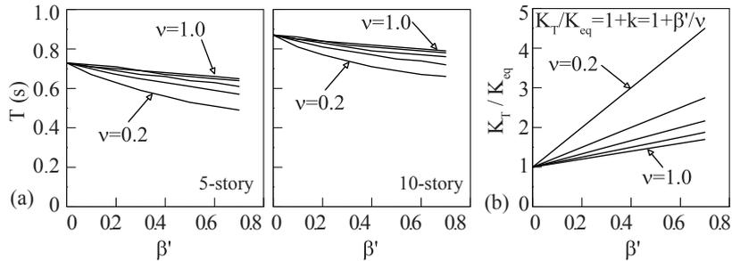
**Figure 2.4.** Influence of damper installation on: (a) natural period  $T$  and (b) total stiffness  $K_T$
