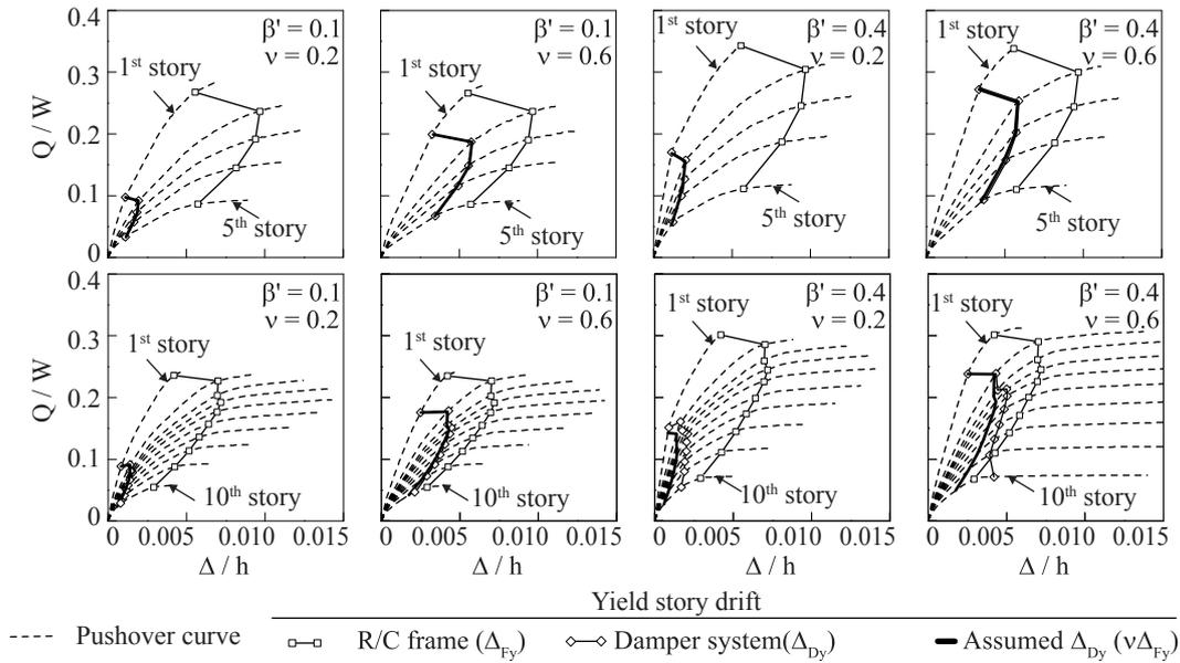
Figure 4.1. Pushover curves after damper installation
