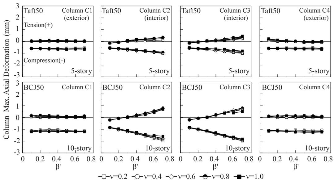
Figure 4.2. First story column maximum axial deformation
