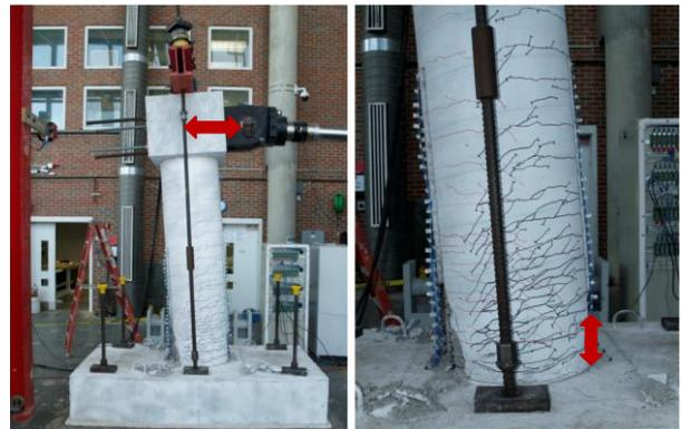
**Figure 10.** Locations of displacement measurement and associated strain measurement (red arrow)
