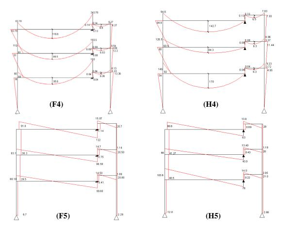
Figure 6. (F4-H4) Moments under lateral load, (F5-H5) Shear forces under lateral load
