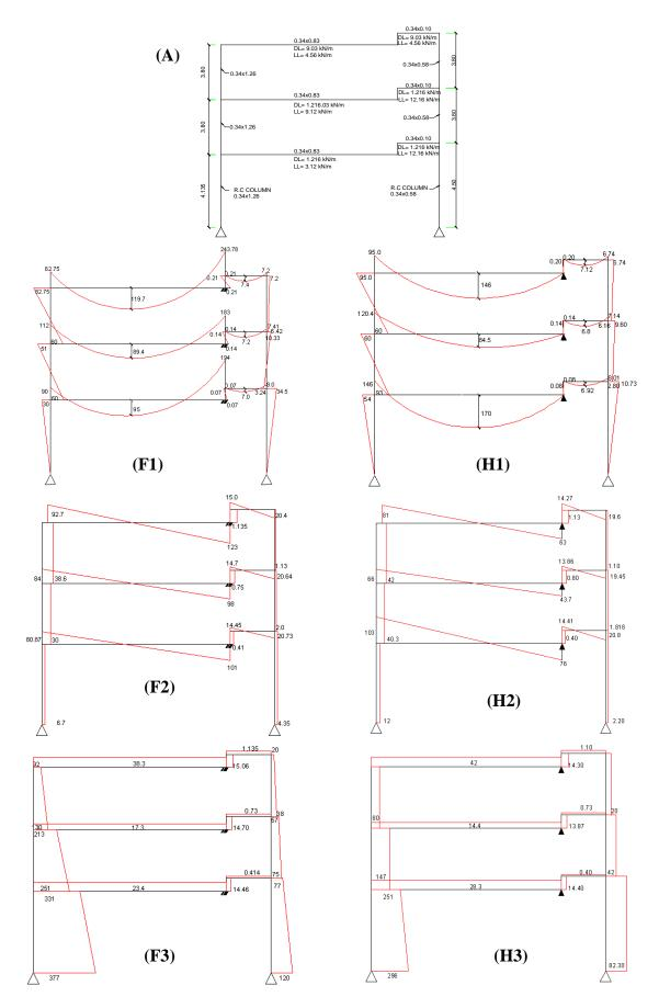
**Figure 5.** (A) Loading diagram, (F1-H1) Moments under gravity, (F2-H2) Shear forces under gravity load, (F3-H3) Axial forces under gravity load (Note: F-fixed, H-hinged)
