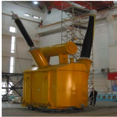
(a) Transformer on shaking table
