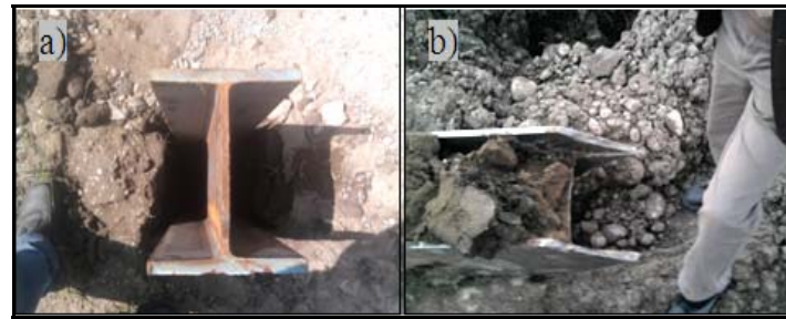
Figure 3.4. a) The plan view of just driven HEB360 in soil. b) The taper shaped end of the HEB360 pile.
