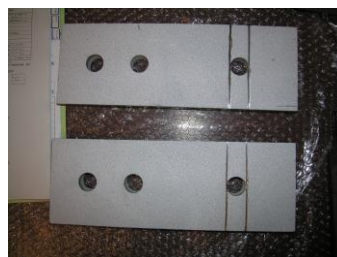
Figure 3.12. Flawed test articles: Direction orthogonal to force application
