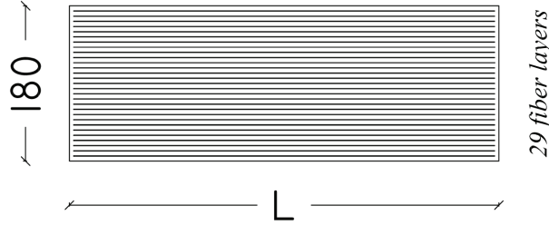
Figure 2.1 Cross section of a bearing
