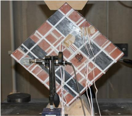
(b) Test setup of CFRP+PP-band retrofitted wallet of diagonal compression test
