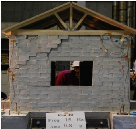
a) Shake table test of 1/4-scale non-retrofitted masonry house
