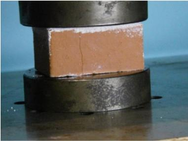
(a) Setup of brick compression test
