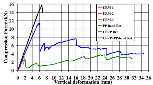
(d) Load-displacement curves of non-retrofitted, PP-band retrofitted, CFRP retrofitted and CFRP+PP-band retrofitted wallets
