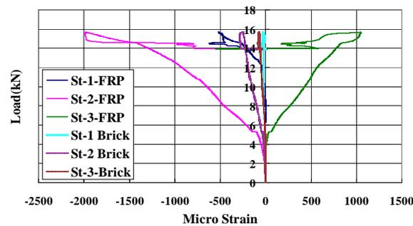
(e) Strain distribution of CFRP retrofitted wallet
