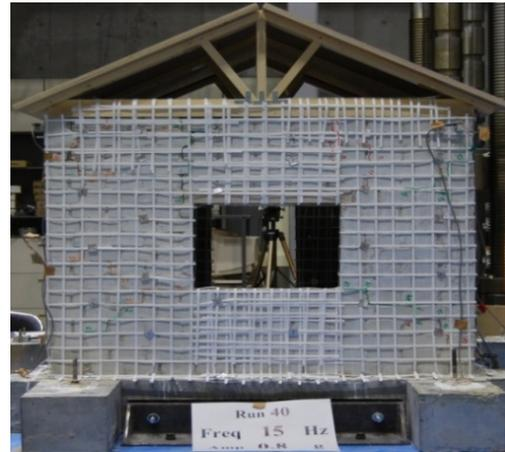
(b) Shake table test of 1/4-scale PP-band retrofitted masonry house
