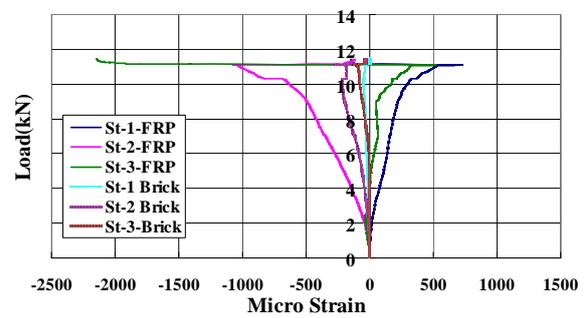
(f) Strain distribution of CFRP+PP-band retrofitted wallet
