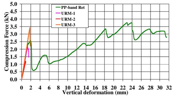
(b) Load-displacement curves of non-retrofitted and PP-band retrofitted wallets
