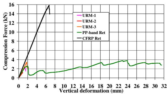
(c) Load-displacement curves of non-retrofitted, PP-band retrofitted and CFRP retrofitted wallets
