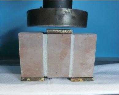
(c) Setup of direct shear test
