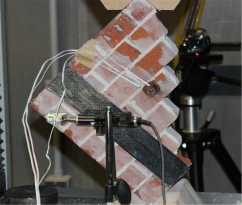
(a) Failure and crack patterns of CFRP retrofitted wallet under diagonal compression
