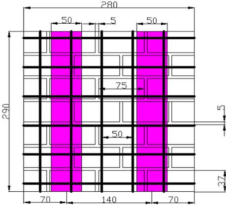
(c) Details of CFRP+PP-band retrofitted wallet
