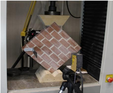
(a) Test setup of non-retrofitted wallet of diagonal compression test
