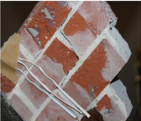
(c) Debonding of CFRP from brick surface crack patterns of CFRP retrofitted wallet
