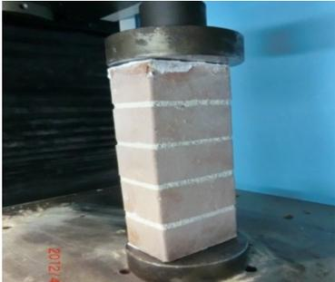
(e) Setup of compression test of masonry of prism
