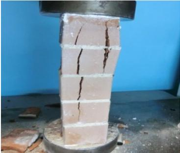
(f) Crack patterns of masonry prisms
