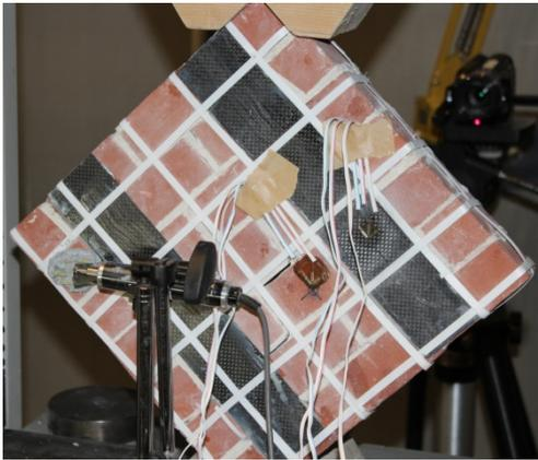
(b) Failure and crack patterns of CFRP+PP retrofitted wallet under diagonal compression
