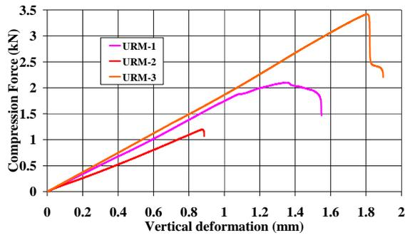
(a) Load-displacement curves of non-retrofitted wallets
