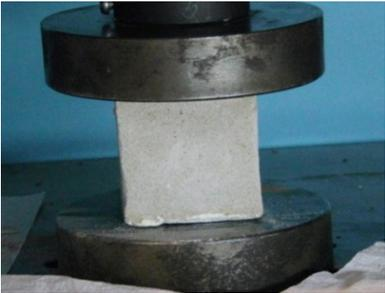
(b) Setup of mortar cube compression test
