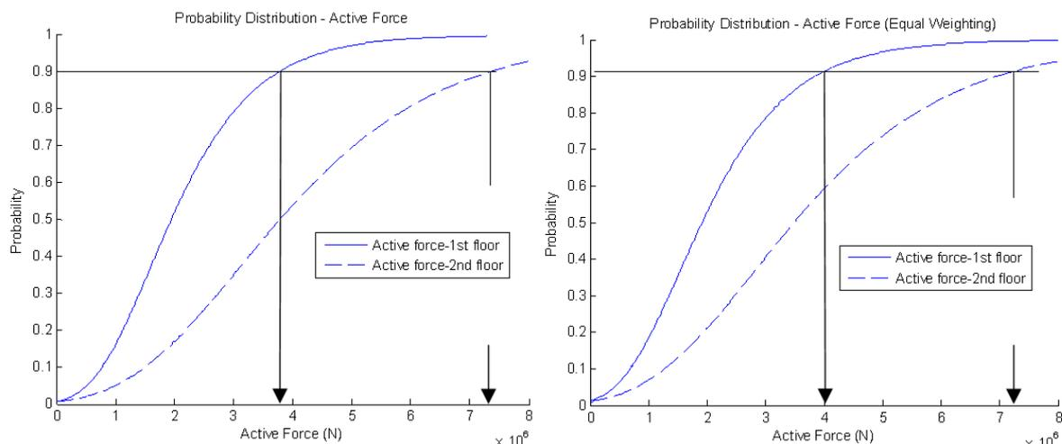
**Figure 4.6.** a) Control force probability by roof weighting b) Control force probability by equal weighting
