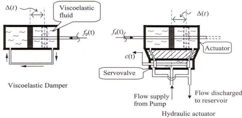
**Figure 2.1.** Hybrid control system: viscoelastic damper plus hydraulic actuator
