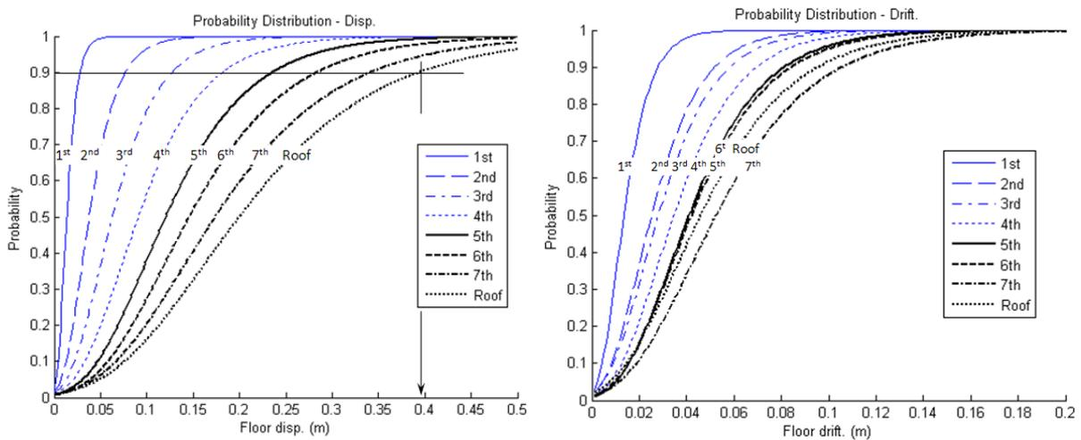
Figure 4.2. a) Response probability - floor displacement b) Response probability - story drift
