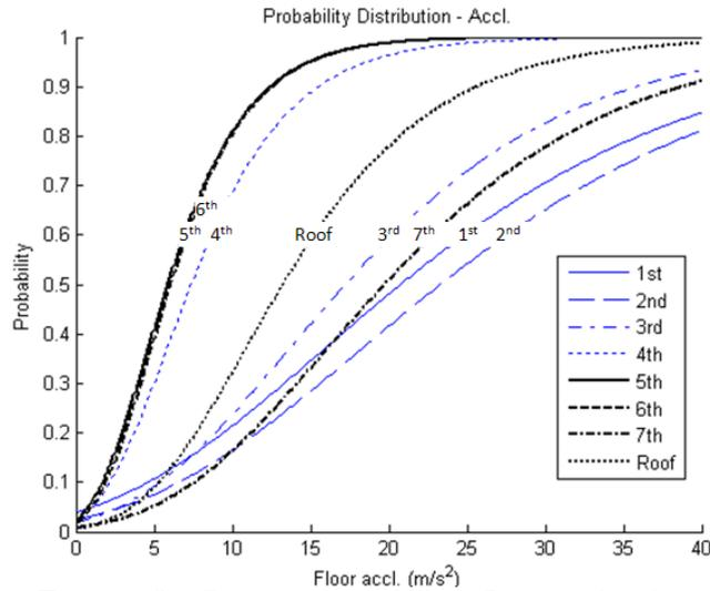
**Figure 4.3.** Response probability - floor acceleration
