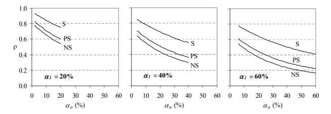
Figure 3.5. Proposed equations of the opening reduction factor
