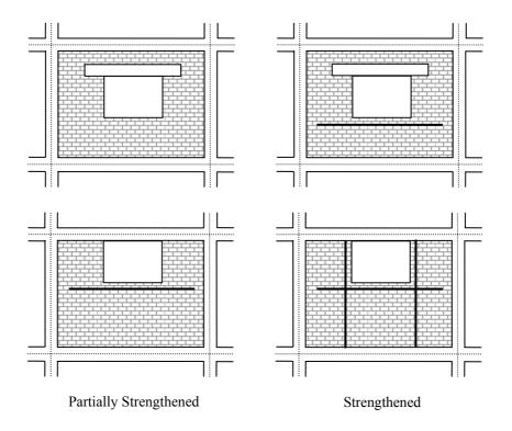
Figure 3.2. Examples of strengthening around opening
