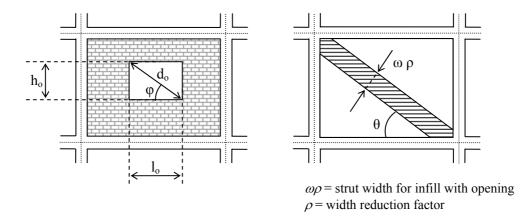
Figure 2.2. Diagonal strut model for infill with opening.
