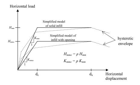
Figure 3.3. Example of strengthening around opening
