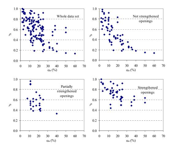
Figure 3.4. Reduction factor evaluated from experimental and numerical analyses
