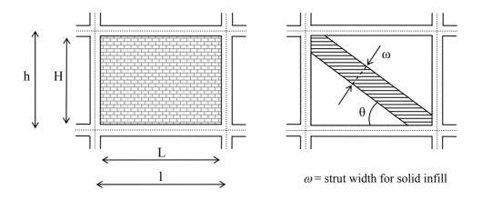
Figure 2.1. Diagonal strut model.
