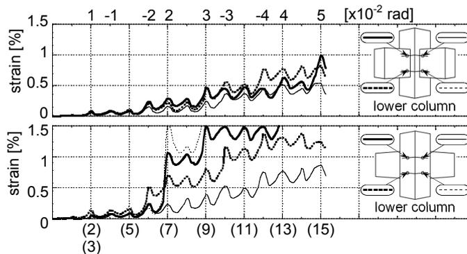
**Figure 3.3.** Strains of Shear Reinforcements in Joint [EXJ-D1]
