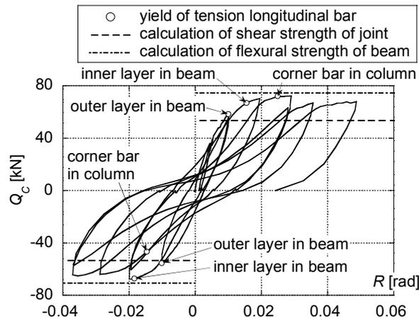
**Figure 3.1.** Shear Load on Column – Story Drift Curve [EXJ-D1]
