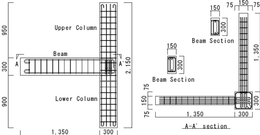
Figure 2.1. Dimension of Specimen [EXJ-D3 for bar arrangements]
