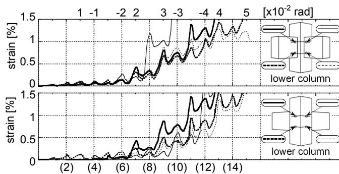
Figure 3.6. Strains of Shear Reinforcements in Joint [EXJ-D2]
