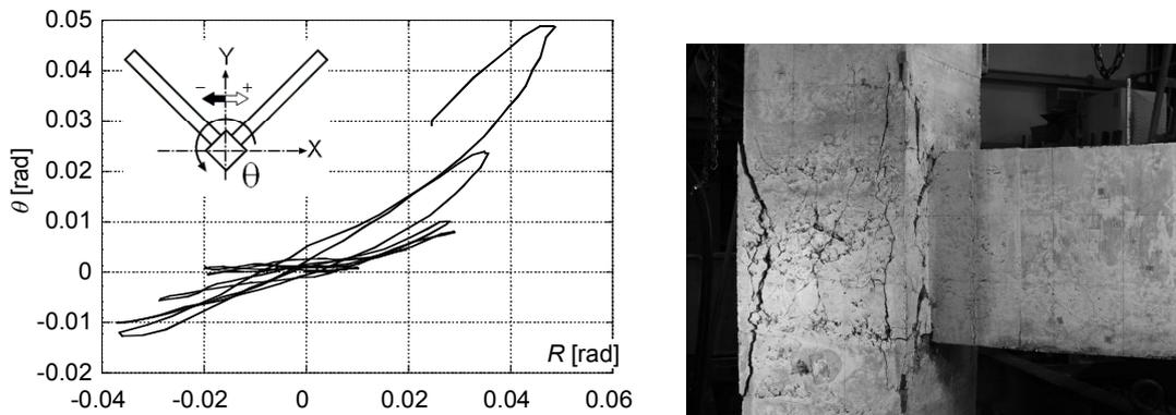
**Figure 3.2.** Rotation around Column Axis and Photo after the Test [EXJ-D1]
