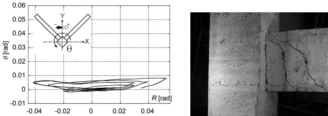
Figure 3.8. Rotation around Column Axis and Photo after the Test [EXJ-D3]
