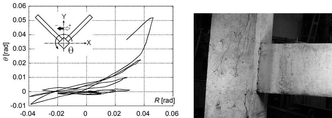
Figure 3.5. Rotation around Column Axis and Photo after the Test [EXJ-D2]
