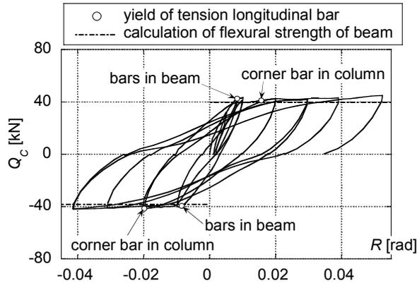
Figure 3.7. Shear Load on Column – Story Drift Curve [EXJ-D3]
