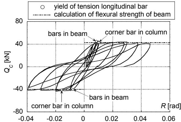
Figure 3.4. Shear Load on Column – Story Drift Curve [EXJ-D2]
