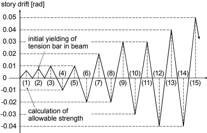
Figure 2.4. Loading Plan
