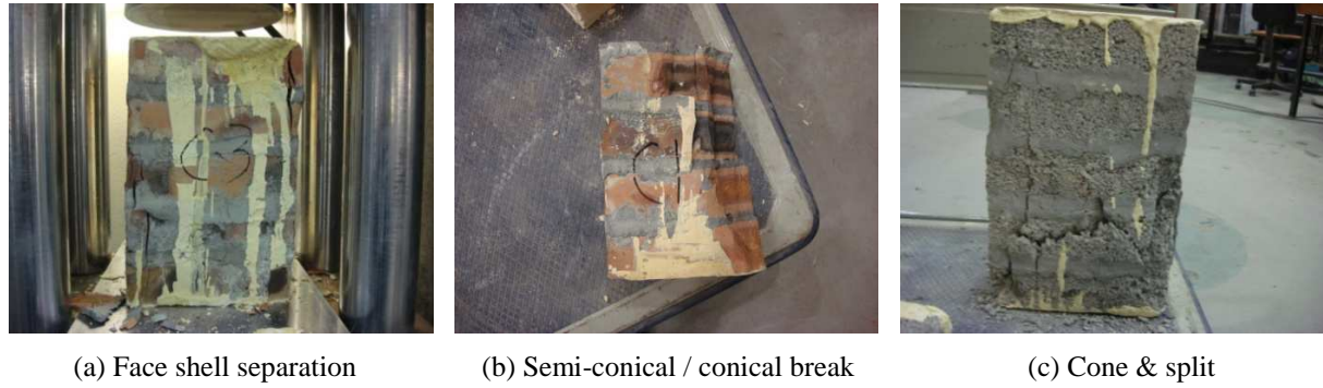
Figure 1. Different failure modes of masonry prisms
