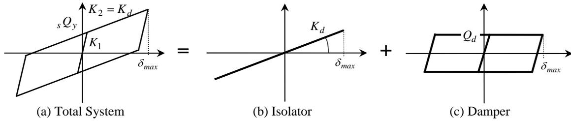
**Figure 6** Restoring Force Characteristic of Analytical Model
