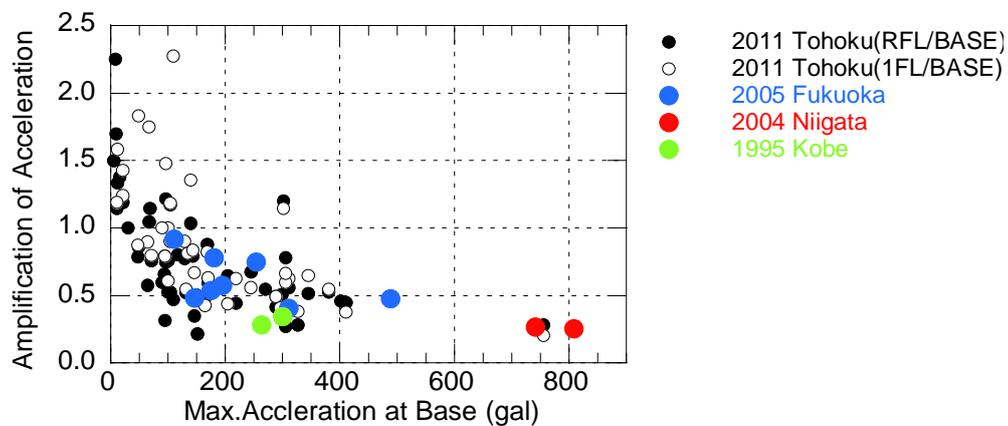
**Figure 2** Amplification Factor of Observed Acceleration of Seismic Isolated Buildings
