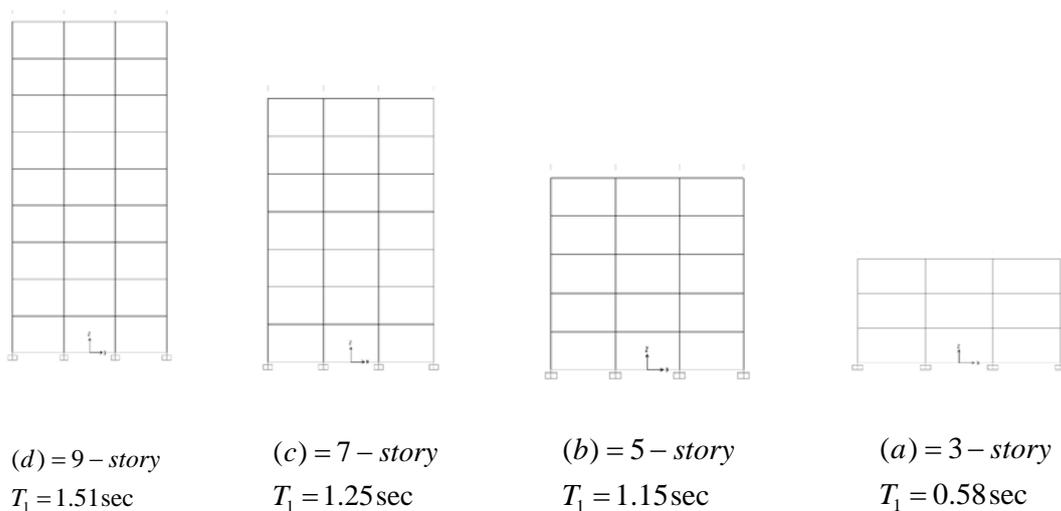
**Figure 1.** Frame elevation view of the structures (3-5-7-9 story buildings)
