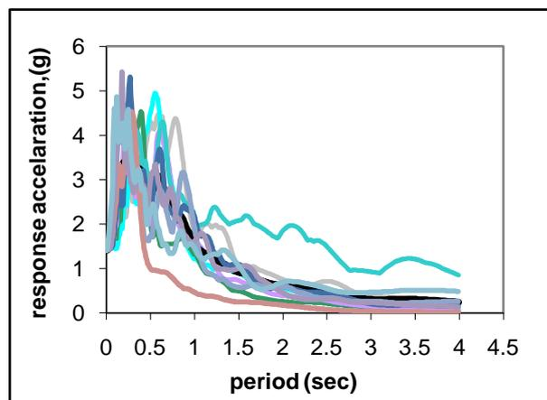
**Figure 2.** (a) Response-acceleration spectra of the set of far-field records of ground motions, damping ratio =5%
