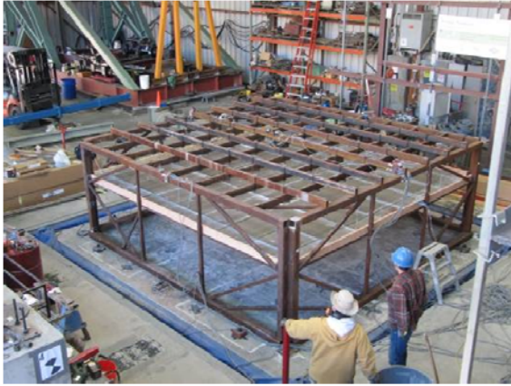
Figure 7. Suspended ceiling system mounted on the test frame prior to experimentation
