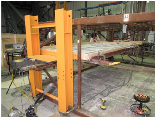
Figure 5. Static test frame and loading frame
