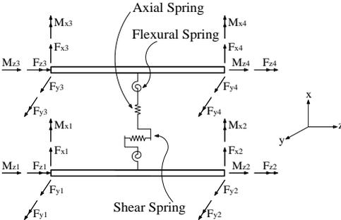
Figure 2. Modeling of staggered walls for pushover analysis
