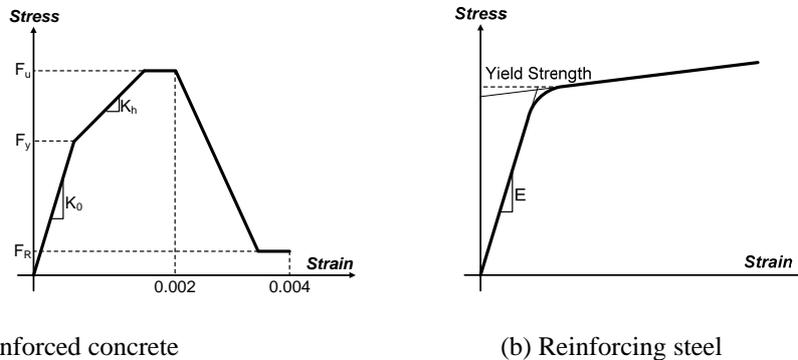
Figure 7. Nonlinear stress-strain relationship of structural materials
