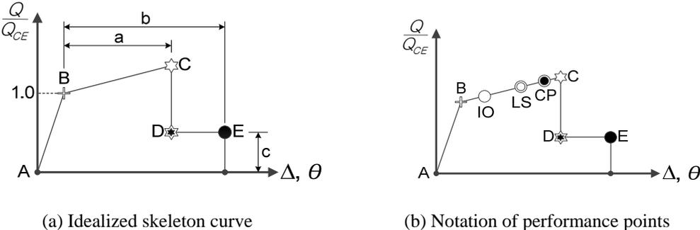
Figure 3. Generalized force-deformation relationship of a RC structural member defined in FEMA 356
