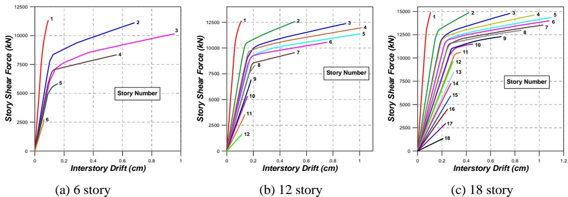
Figure 5. Relationship of story shear vs. inter-story drift
