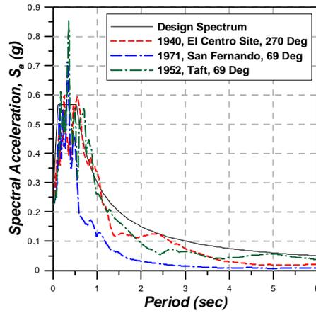
Figure 8. Response spectra of the scaled ground motions
