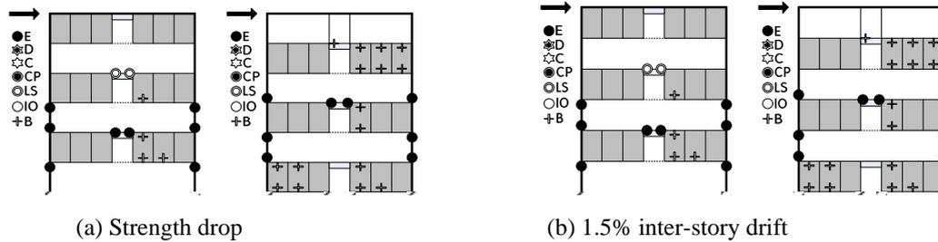
Figure 6. Plastic hinge formation at the points of sudden strength drop and at the 1.5% inter-story drift
