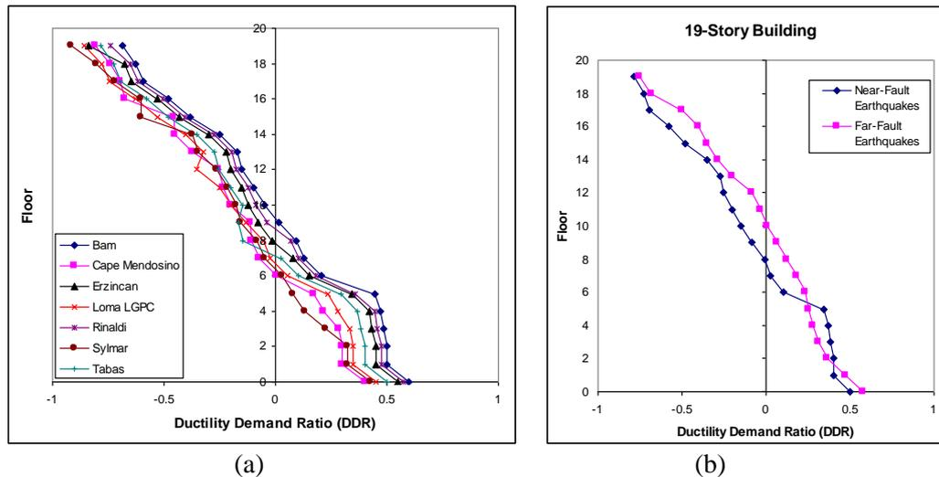
Figure 6. Ductility demand ratios for 19-story buildings (a) near-fault records; (b) mean values
