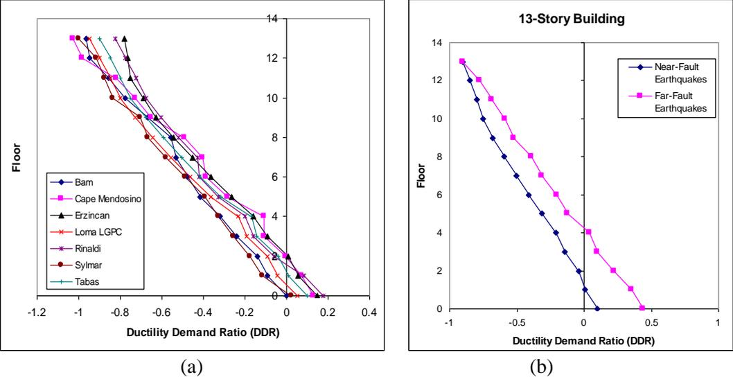
Figure 4. Ductility demand ratios for 13-story buildings (a) near-fault records; (b) mean values
