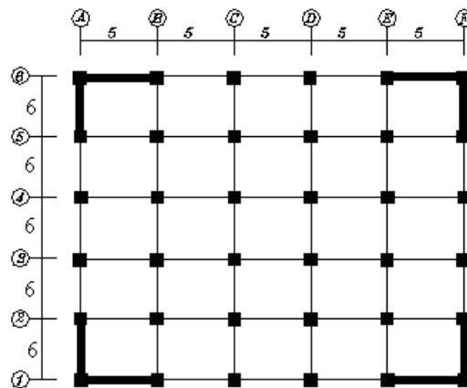
**Figure 2.** Structural configuration of studied buildings (units: meter)
