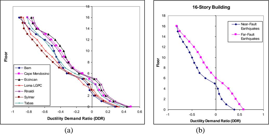
Figure 5. Ductility demand ratios for 16-story buildings (a) near-fault records; (b) mean values
