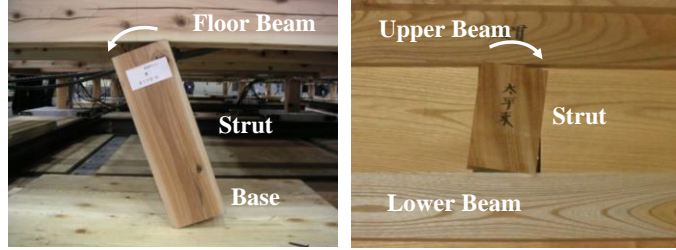
Figure 2.6. Deformation of strut on the base or the beam
