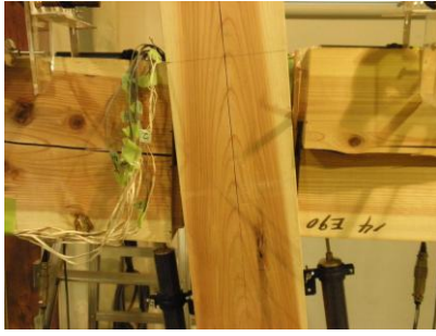
Figure 4.3. Deformed Specimen A-2-2(0.1rad)
