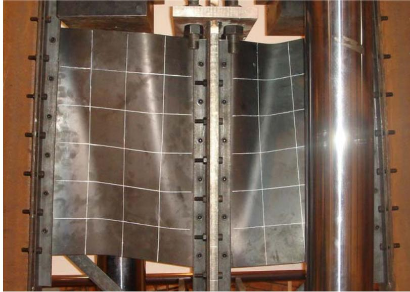
**Figure 6.** The deformed shape of the specimens M4 tested under monotonic loading with zero friction and no slot effects.
