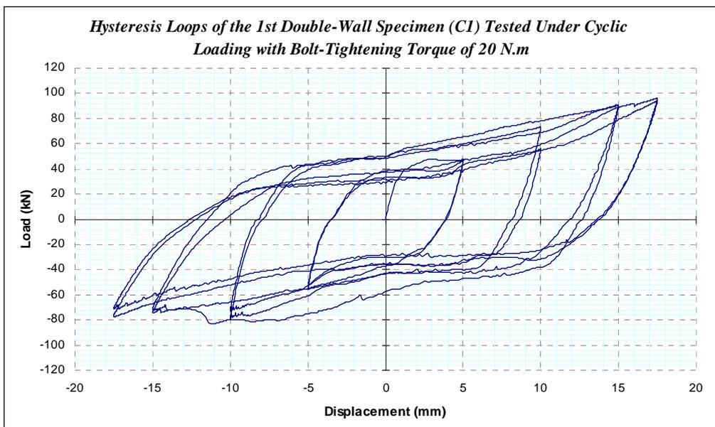
**Figure 8.** Hysteresis Loops of the 1st double-wall specimen (C1) tested under cyclic loading.
