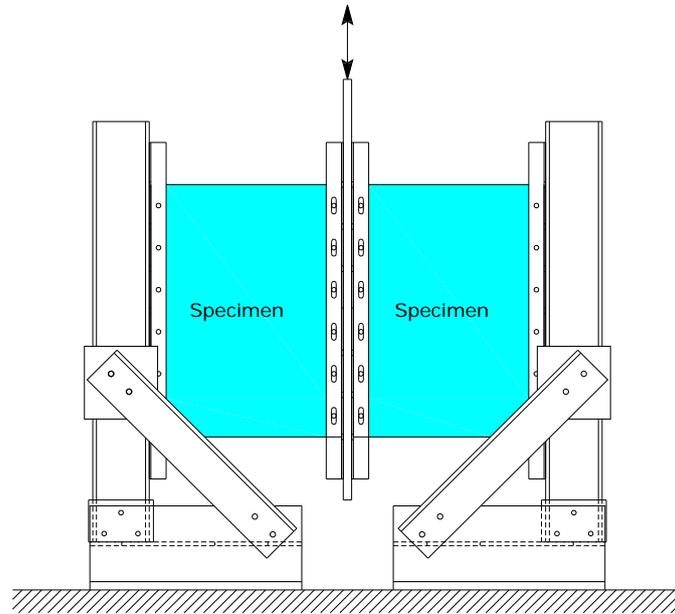
**Figure 2.** Schematic drawing of the test assembly with 2 specimens of Type 2 (with slots at one side and bolt holes at the other) mounted on it.
