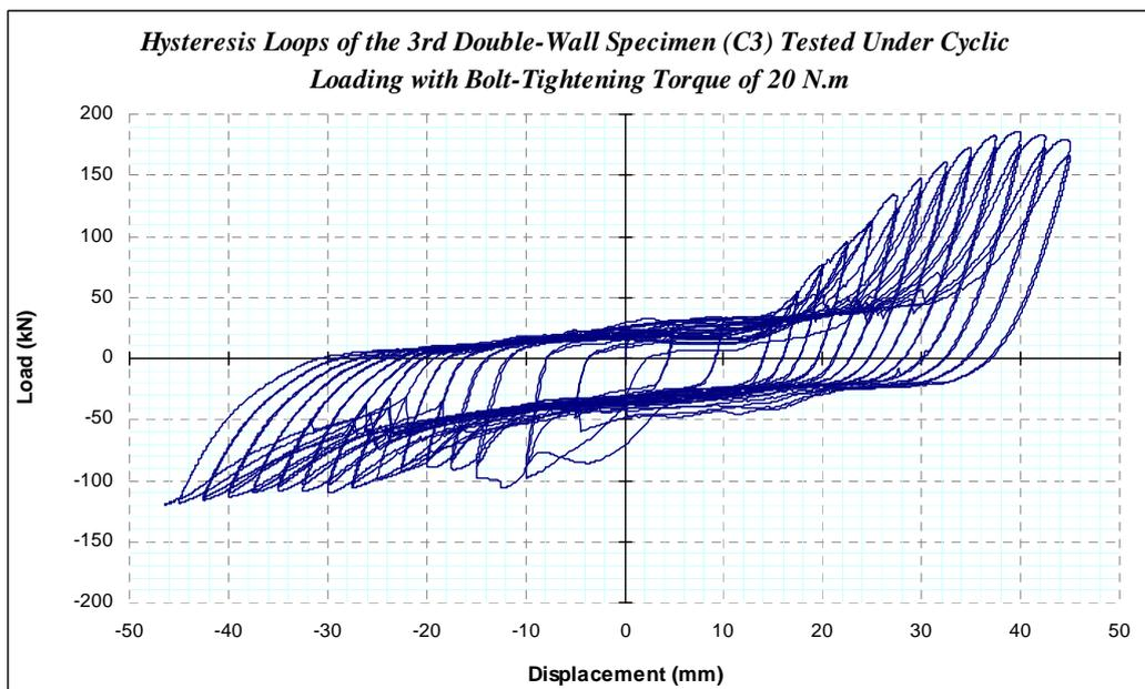
**Figure 10.** Hysteresis Loops of the 3rd double-wall (with BSPs) specimen (C3) tested under cyclic loading.
