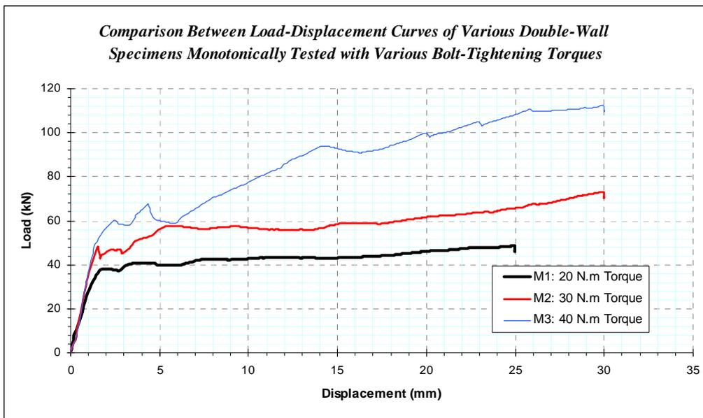
**Figure 4.** Load-Displacement curves of three monotonically-tested double-wall specimens with different bolt-tightening torques of 20, 30 and 40 N.m.
