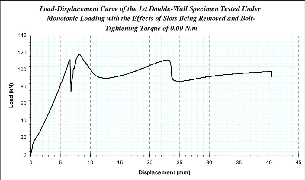
**Figure 5.** Load-Displacement curve of a monotonically-tested double-wall specimen with zero friction and no slots effects (M4 specimens).
