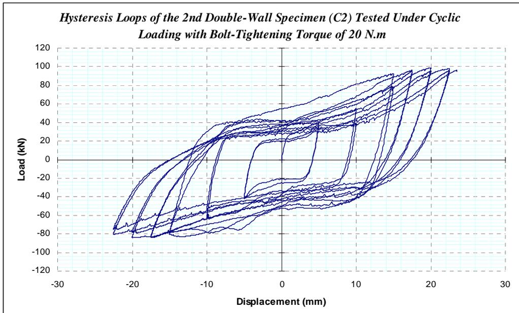
**Figure 9.** Hysteresis Loops of the 2nd double-wall specimen (C2) tested under cyclic loading.
