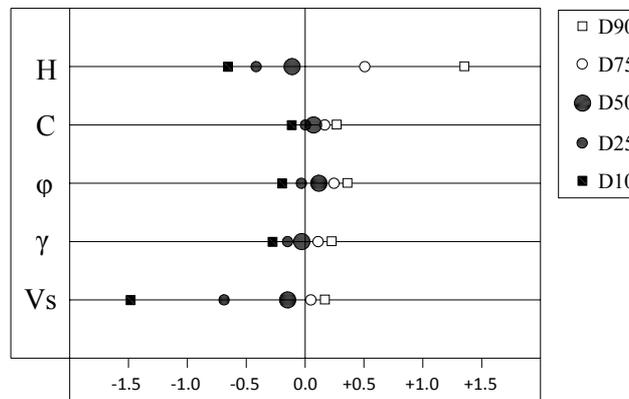
**Figure 5.1.** Sensitivity analysis of AF related to input domain
