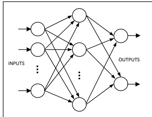
**Figure 3.1.** A multi-layer feed forward neural network with three layers
