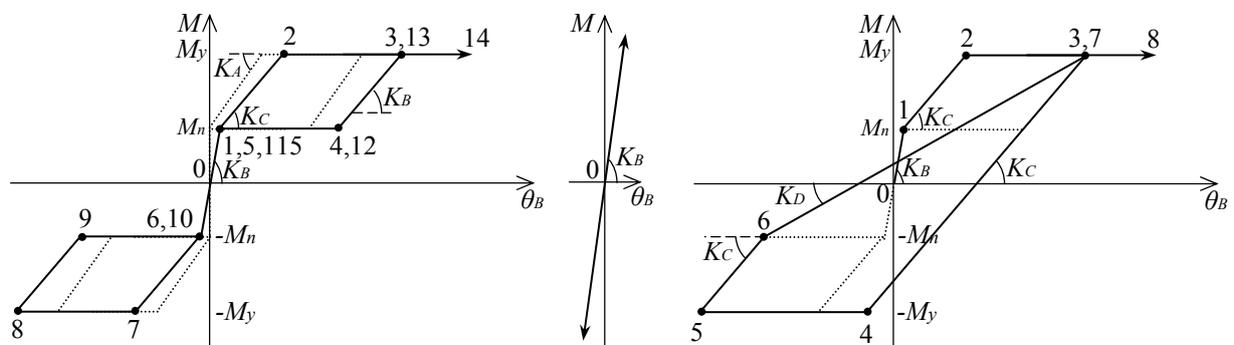
(a) Rotation angle of Column Base (Model A)
