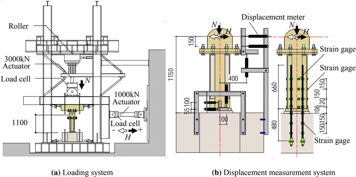
**Figure 2.2.** Test setup system (unit:mm)
