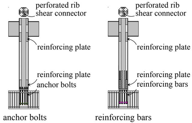
Figure 1.2. Column with column base
