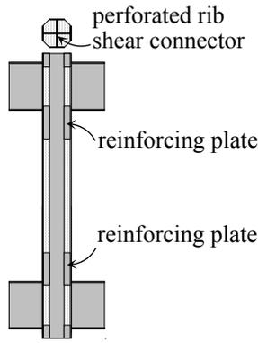
Figure 1.1. Column without column base
