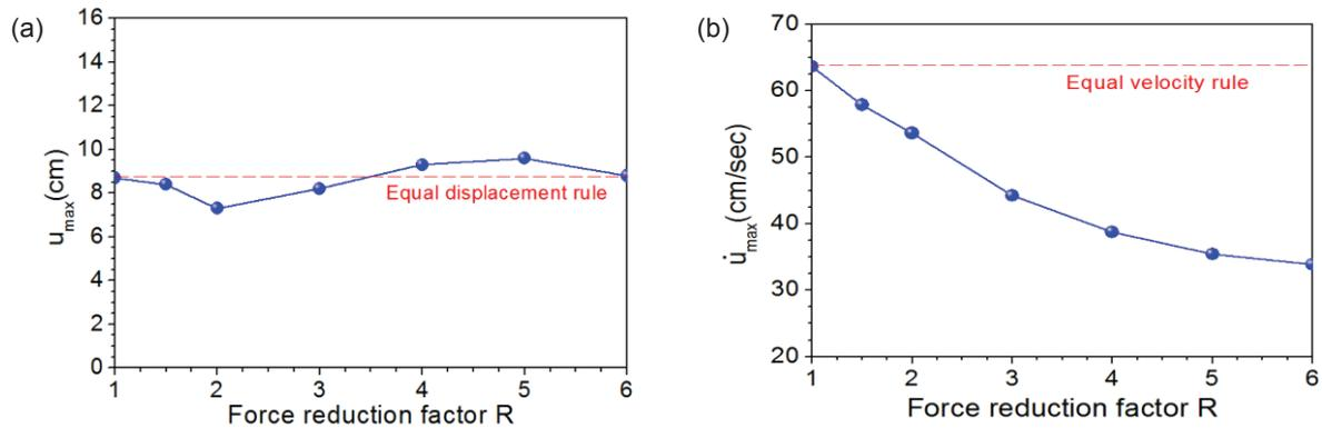
Figure 2. (a) Maximum displacement, and (b) maximum velocity
