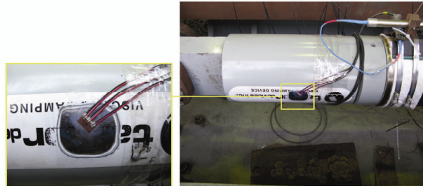
Figure 5. Strain-gauge rosette on the extender of the 1100-kN damper
