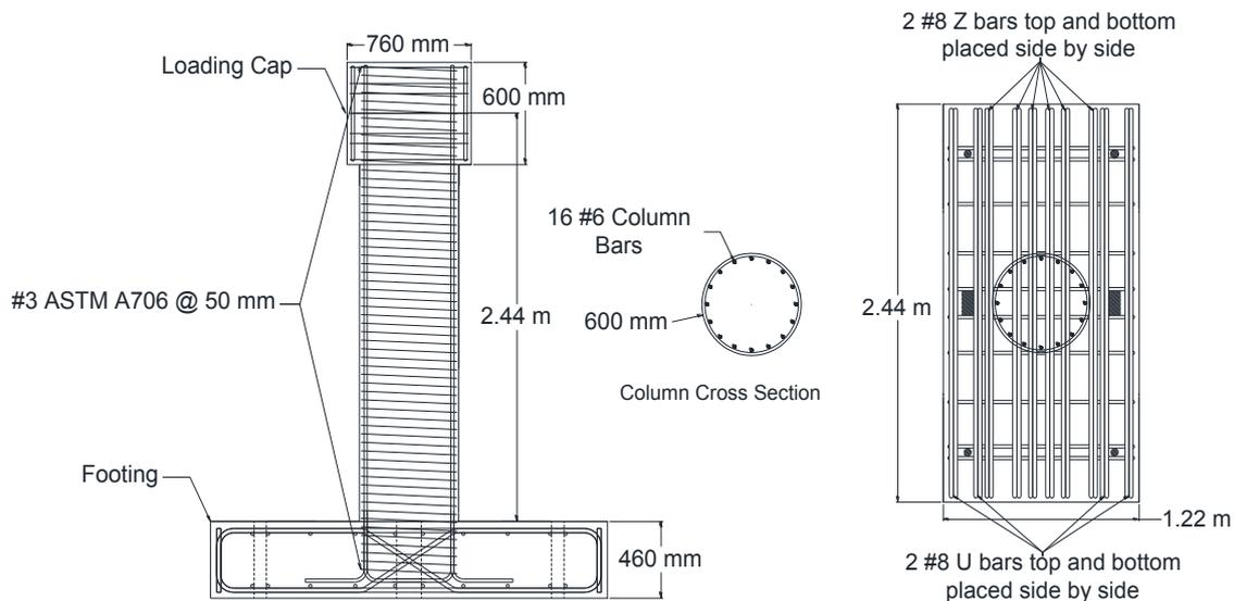
**Figure 2.2.** Column specimen reinforcement details
