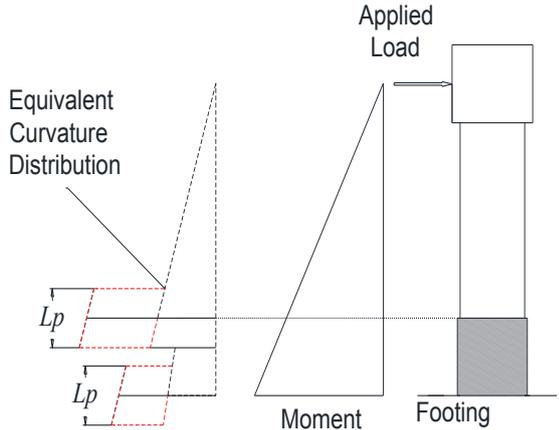
Figure 4.2. Modified plastic hinge method
