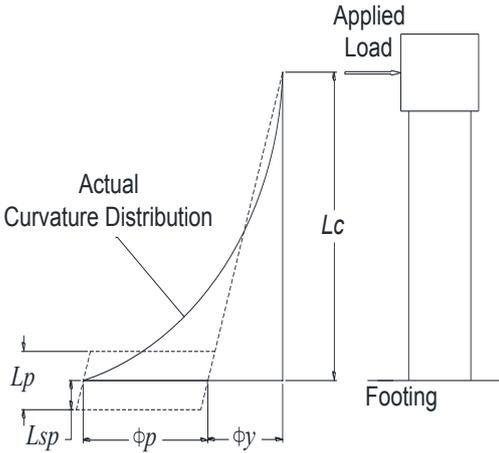
Figure 4.1. Plastic hinge method
