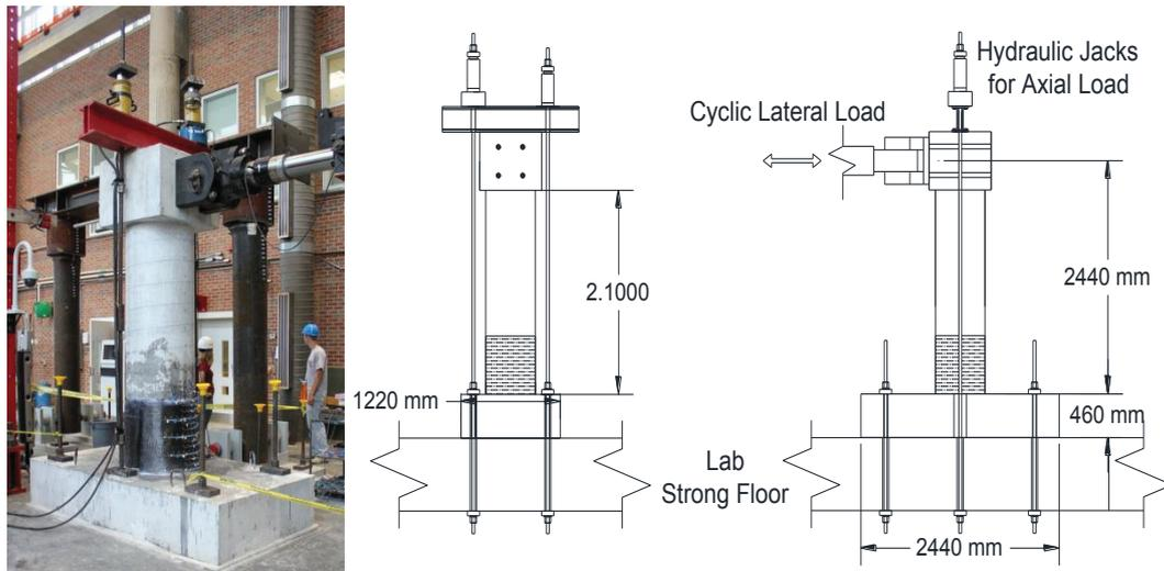
**Figure 2.5.** Column specimen test setup
