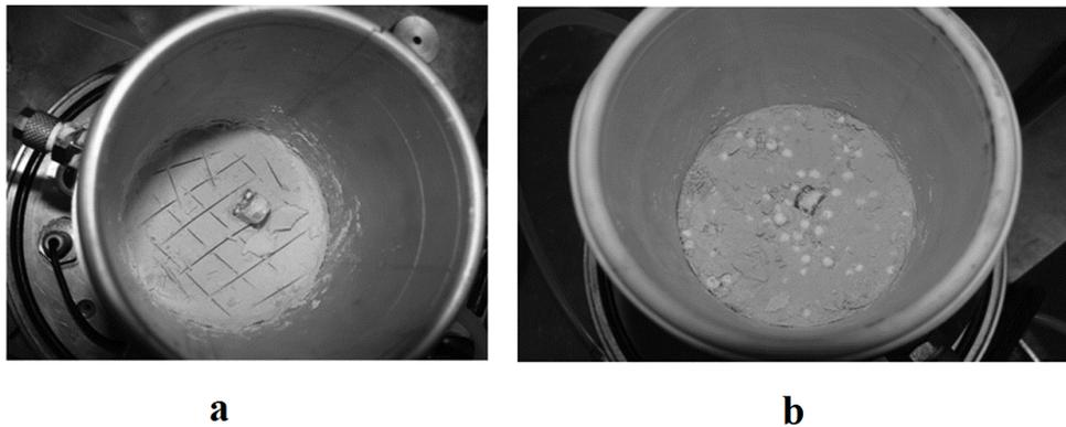
**Figure 1.** Clay specimens for cyclic triaxial test: a) pure clay specimen; b) mixed specimens
