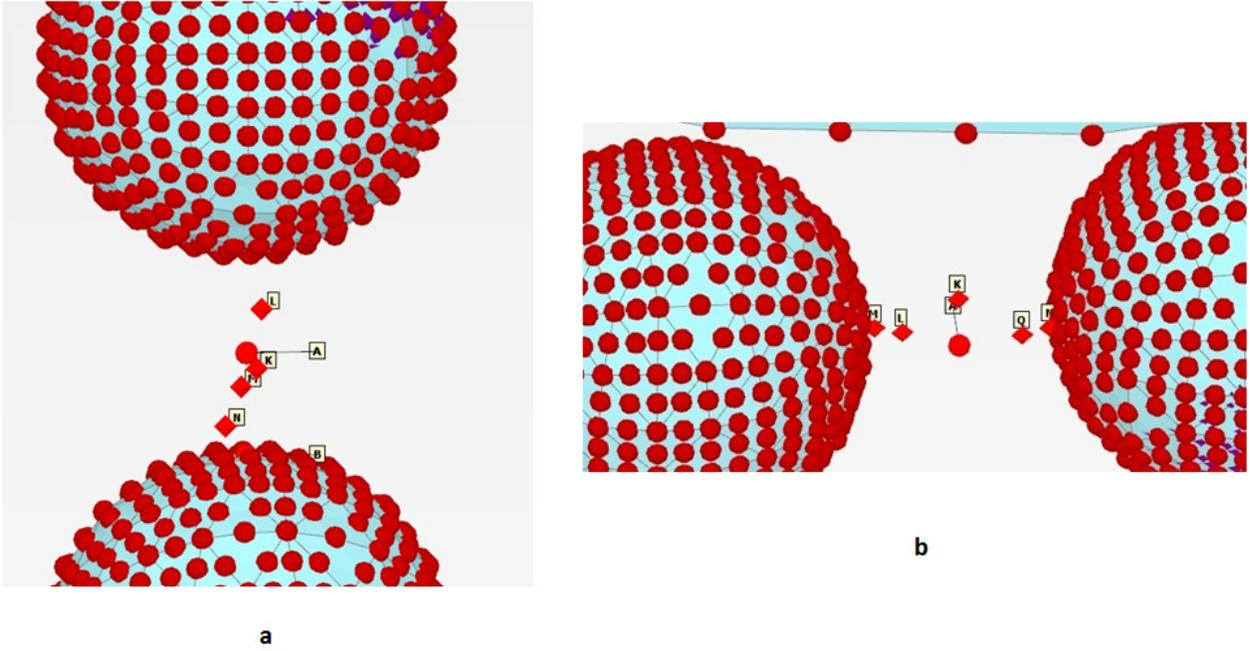
**Figure 4.** Locations of points where volumetric strain change was captured during analyses: a) vertically aligned inclusions, b) Horizontally aligned inclusions
