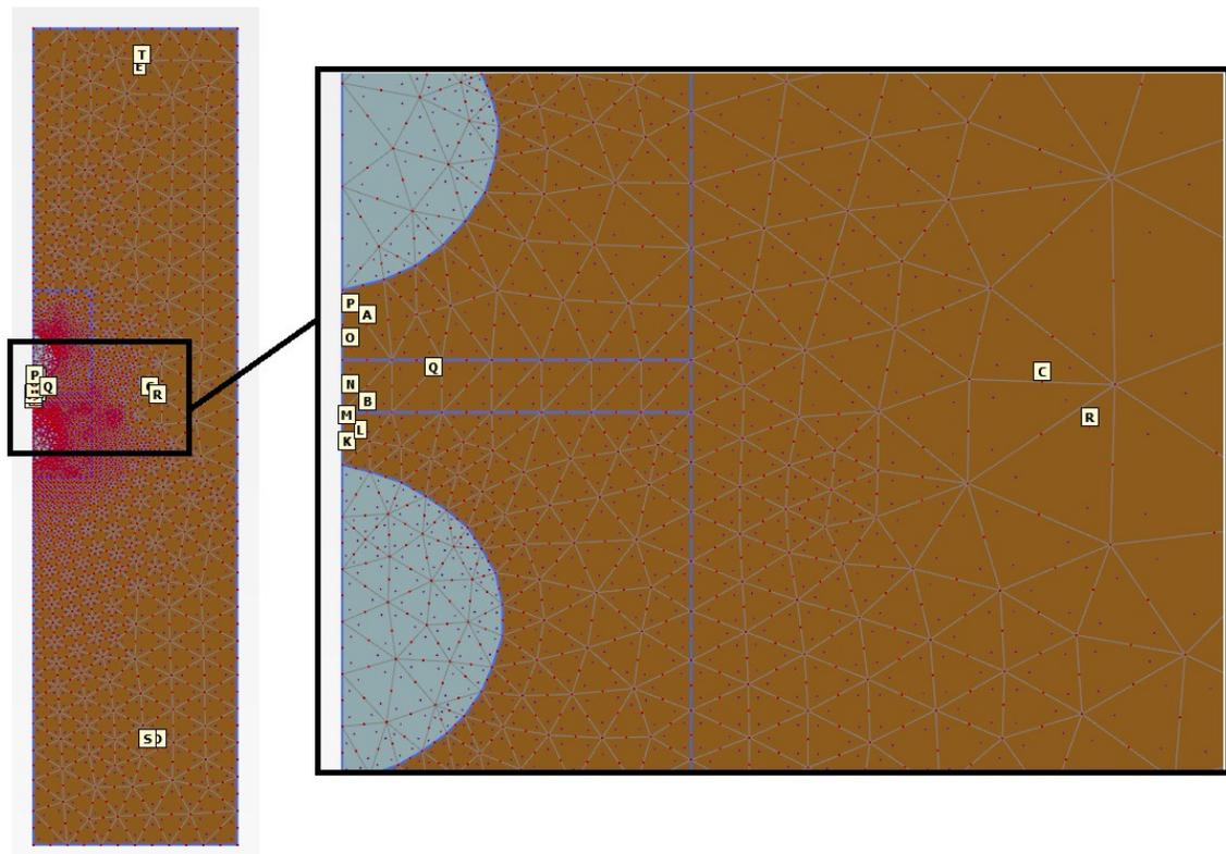
**Figure 6.** Geometry of the 2D axisymmetric model including locations of the observation points at compression path (P, A, ...) and far from inclusions (C, S, ...)
