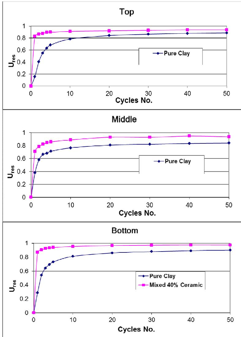
**Figure 2.** Normalized residual excess pore water pressure change with increase of cycles at frequency of 0.005 Hz at a) top; b) middle; c) bottom of the specimens
