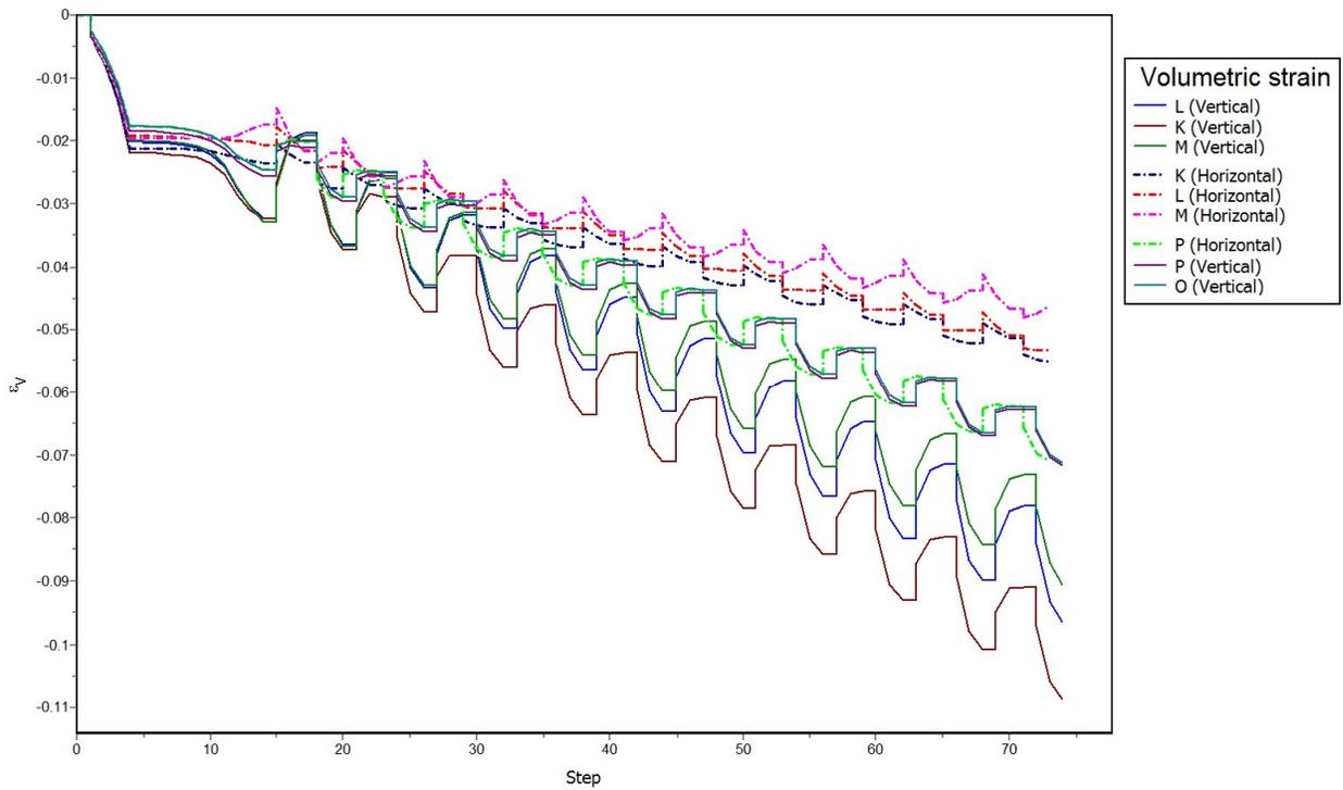
**Figure 5.** Variation of volumetric strain with loading step in areas between inclusions (points L, K and M in vertical and horizontal position, as shown in Fig. 4, and P and O at specimen top and bottom, far from inclusions)
