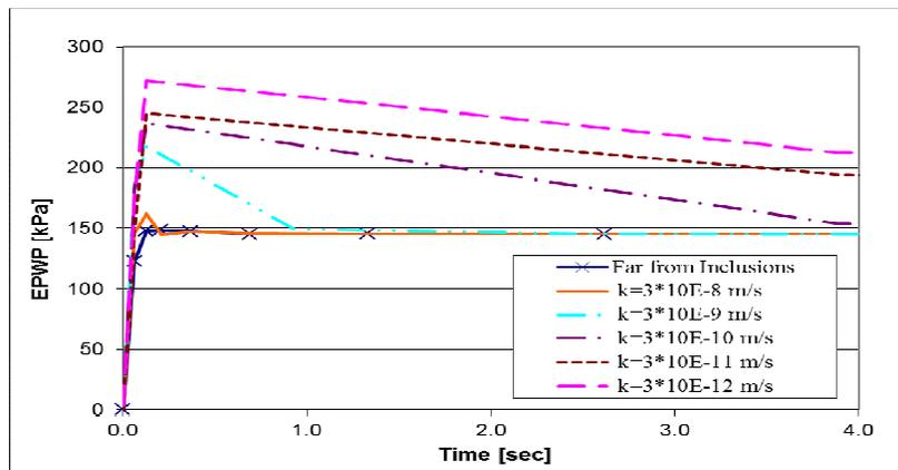
**Figure 8.** Change of excess pore water pressure with time at compression path and far from inclusions inside clay specimen, after 1.5% monotonic strain
