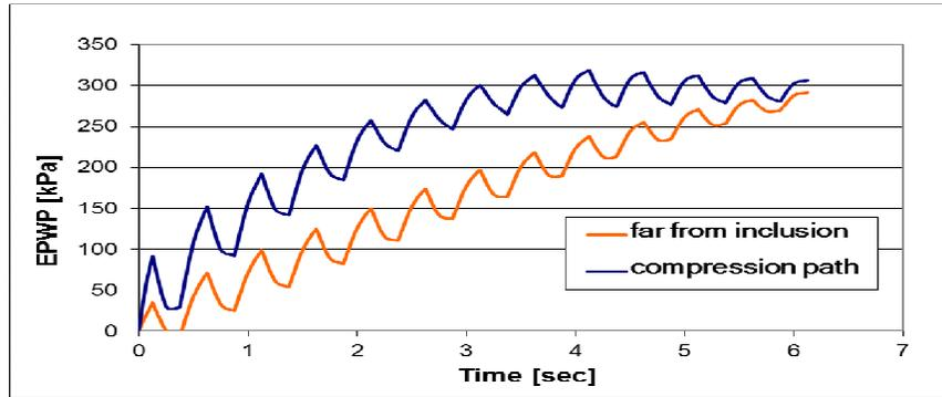
**Figure 7.** Change of excess pore water pressure with time at compression path and far from inclusions ( $k=3 \times 10^{-11}$  m/s,  $f = 2$  Hz)
