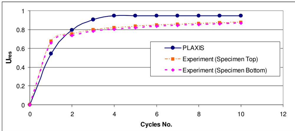
**Figure 3.** Normalized residual excess pore water pressure change with increase of cycles from cyclic triaxial test and those simulated in Plaxis by UBC3D model
