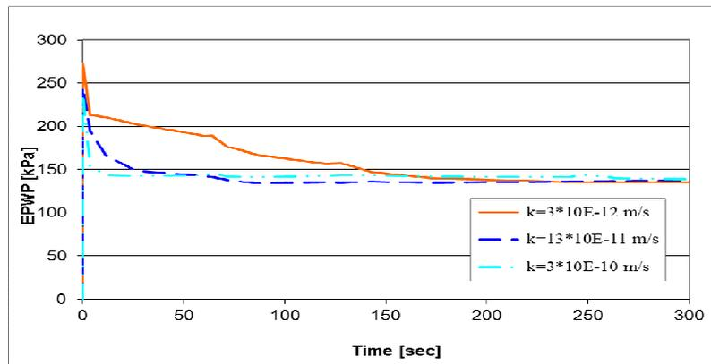
**Figure 9.** Change of excess pore water pressure with time at compression path inside clay specimen, after 1.5% monotonic strain
